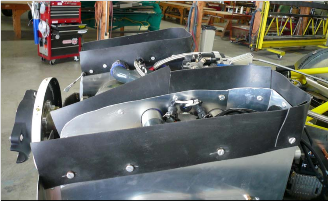
Finished Air Ducts with Baffle Material.
