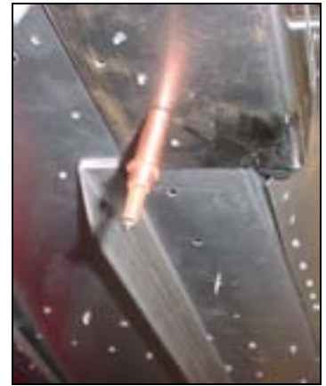
Bottom rivet line through the Floor Channel 6TD3-2 A5 PITCH 30
