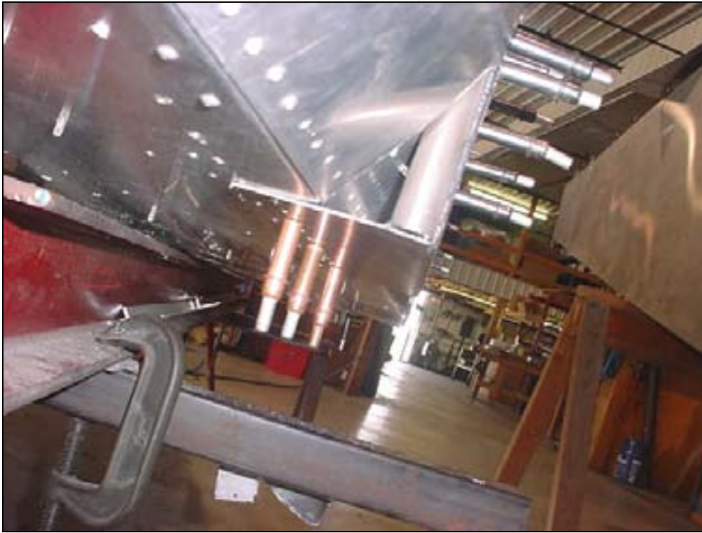
Bottom rivet line through the Floor Channel 6TD3-2 A5 PITCH 30
