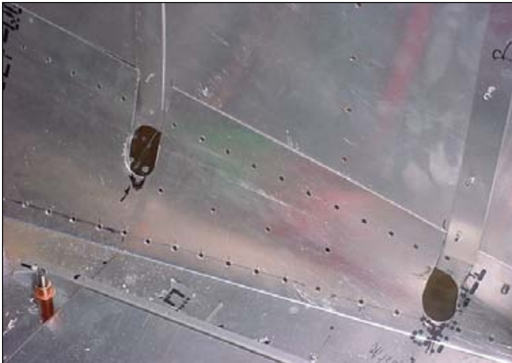
Inside view of right side. Cutout in Cabin Floor Skin 6B10-1, cutout to make room for the tube.
