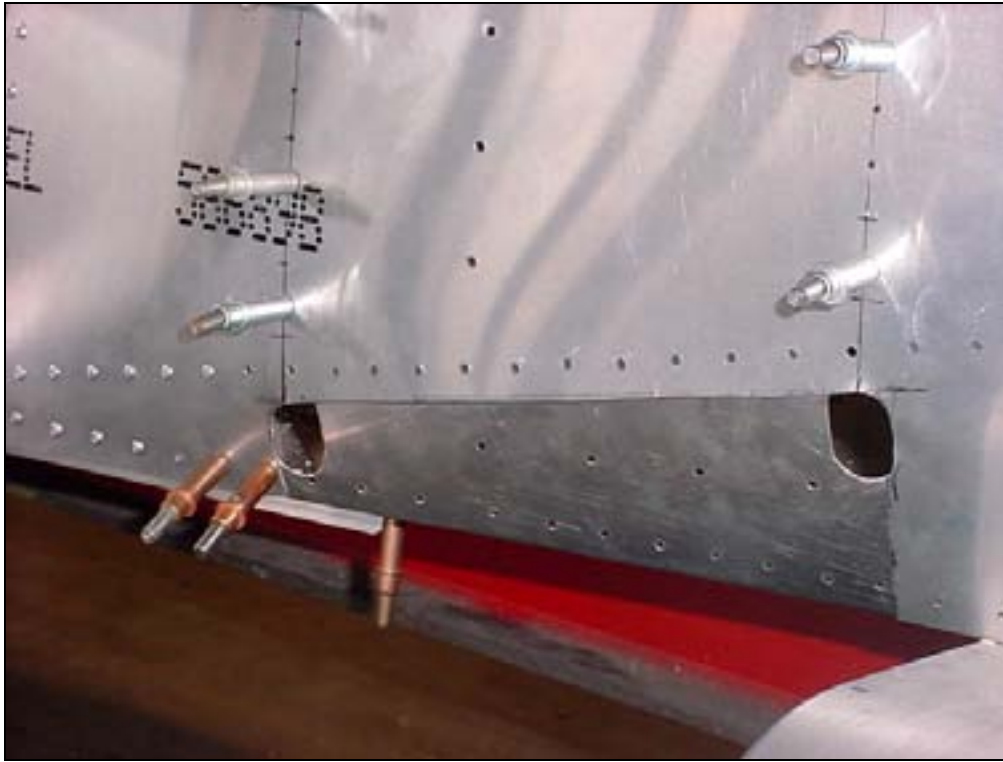
Rectangular cutout in the fuselage Forward Side Skin 6B11-2
