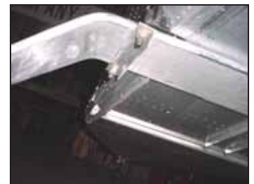
CHECK: the gear is square (90 degrees) to the fuselage center line.
