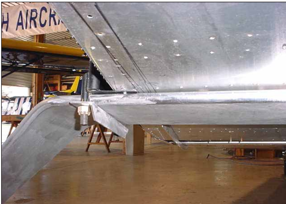
CHECK: the gear is square (90 degrees) to the fuselage center line.
