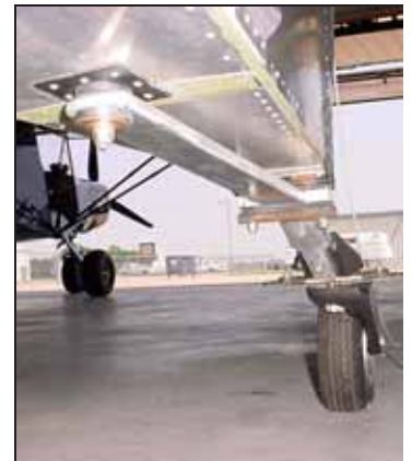
Tail spring underneath fuselage between the front and rear HT frames
