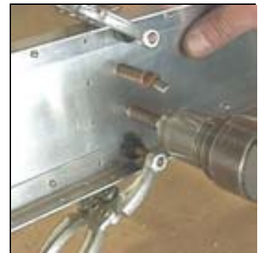
Undersize pilot holes: Drill #30 and cleco.
