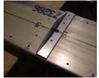
The 1/4" hole on the Hinge Angles is in line with the spar center line
