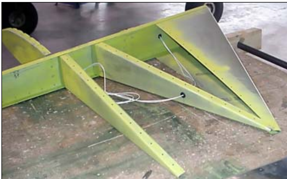
Flanges on the nose rib point down.
