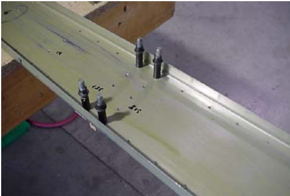
Undersize pilot holes: Drill #30 and cleco.
