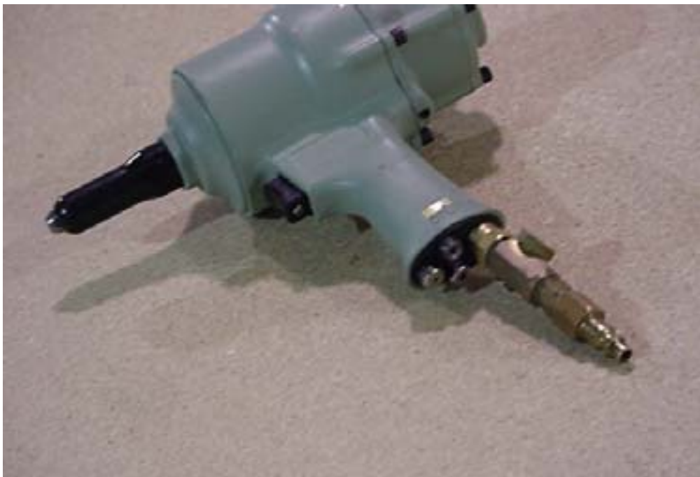
Pneumatic riveter. The A4 and A5 rivets can be pulled with a hand riveter or with a power tool (pneumatic or hydraulic).
