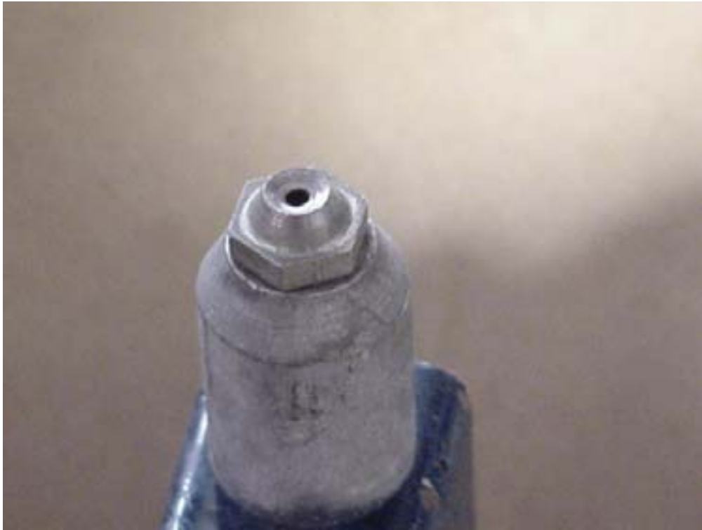
Custom machined nose piece on screwed in the riveter head.
