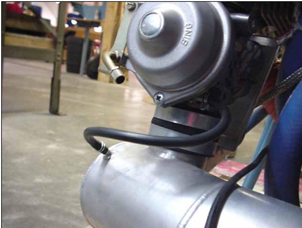
Vent hose connected to air-box bared outlet on the Rotax tuned air-intake box
