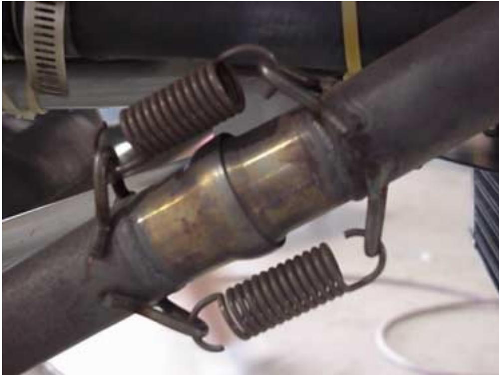
Detail of ball joint with springs
