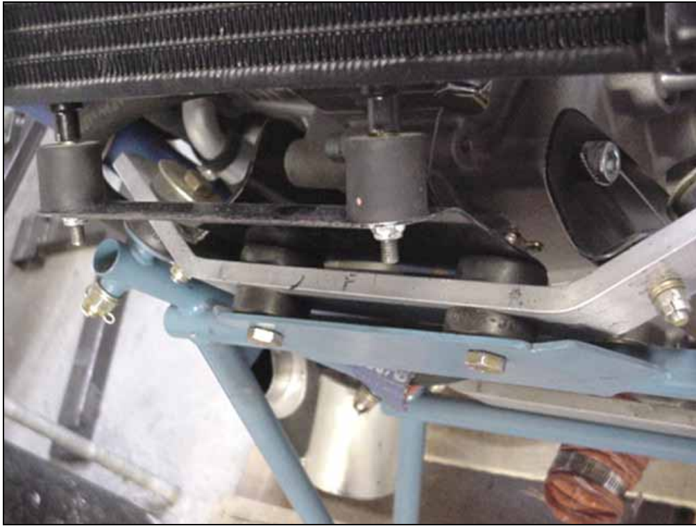
3/8" holes. Bolted on of 22001-13 Green Bot Barry Mounts
