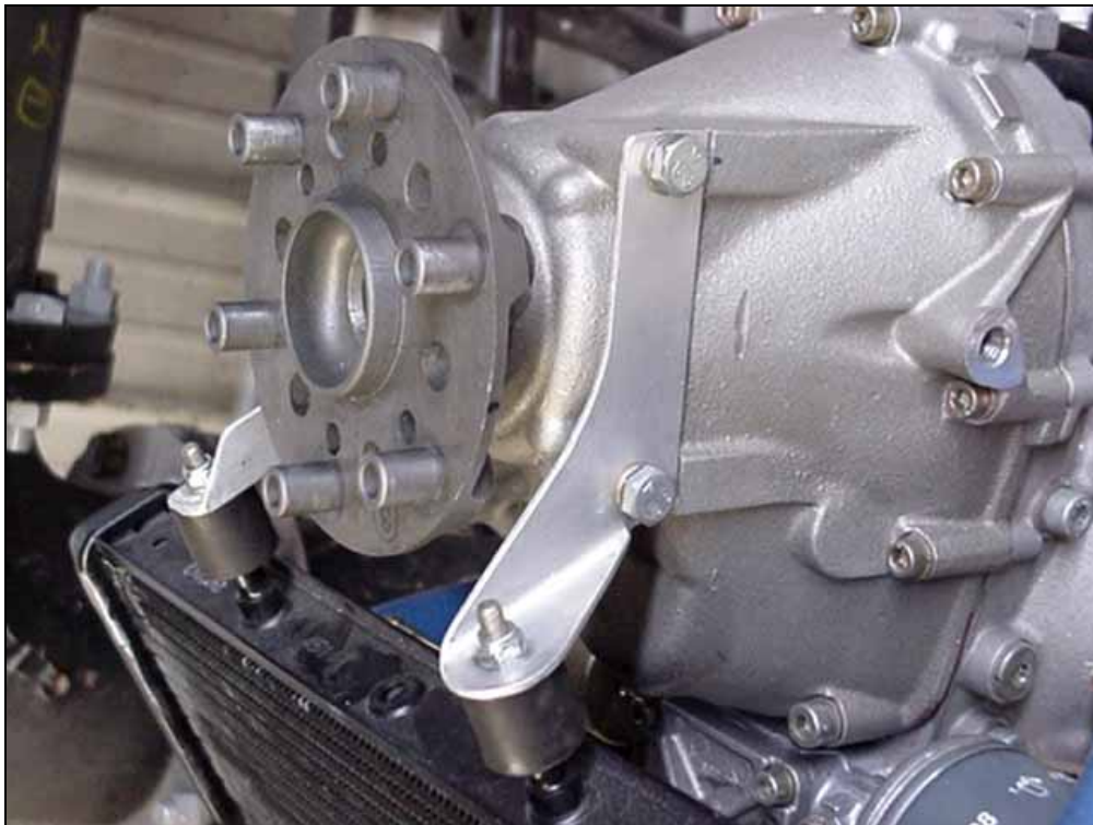
Holes in E1-1X to bolt the engine
