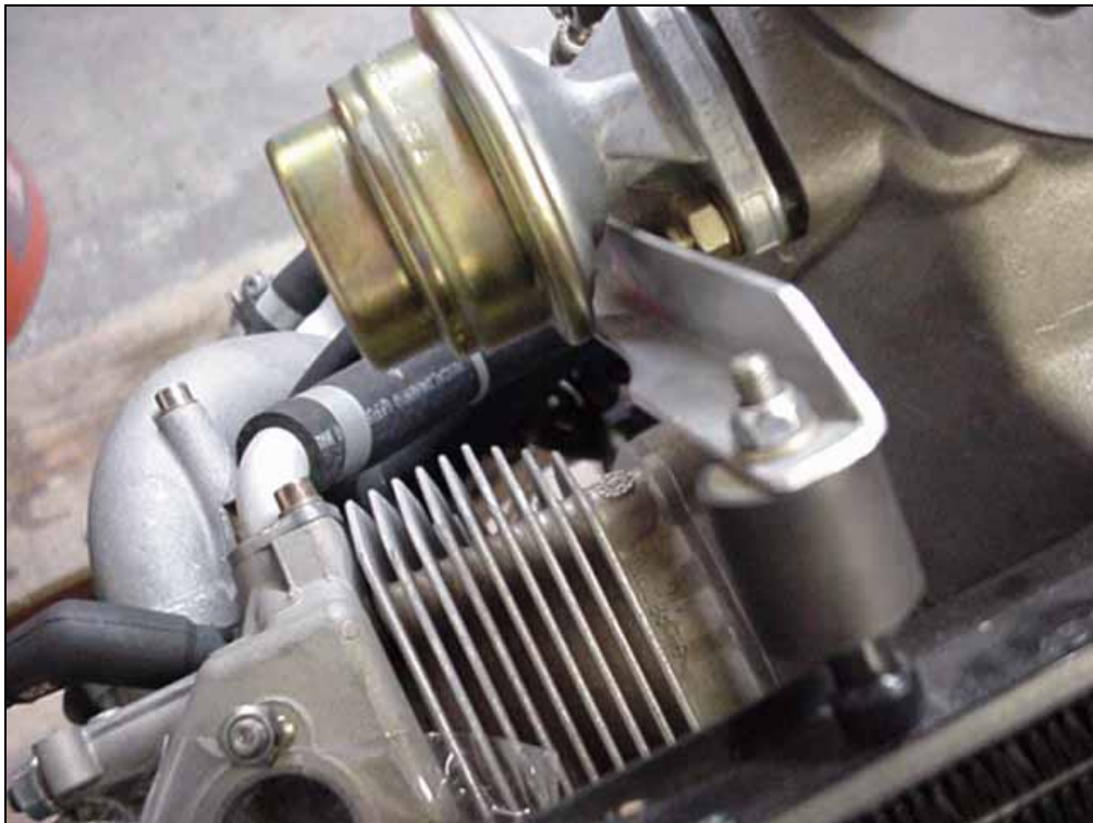
Cutout in bottom flange to make room for the fuel pump
