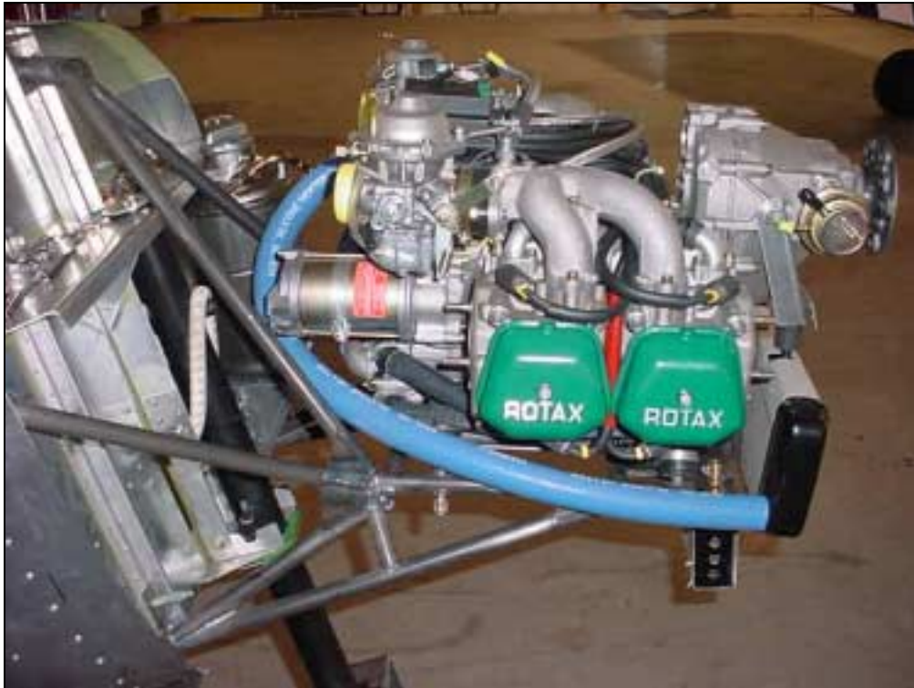
Bottom right of radiator to the pressure reservoir on top of the engine.
