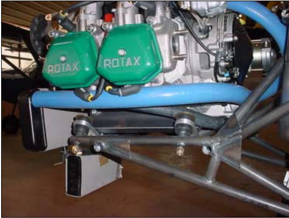
Top left of radiator to water pump.
