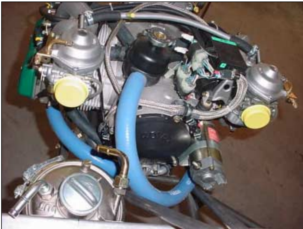
Pressure reservoir on top of engine.
