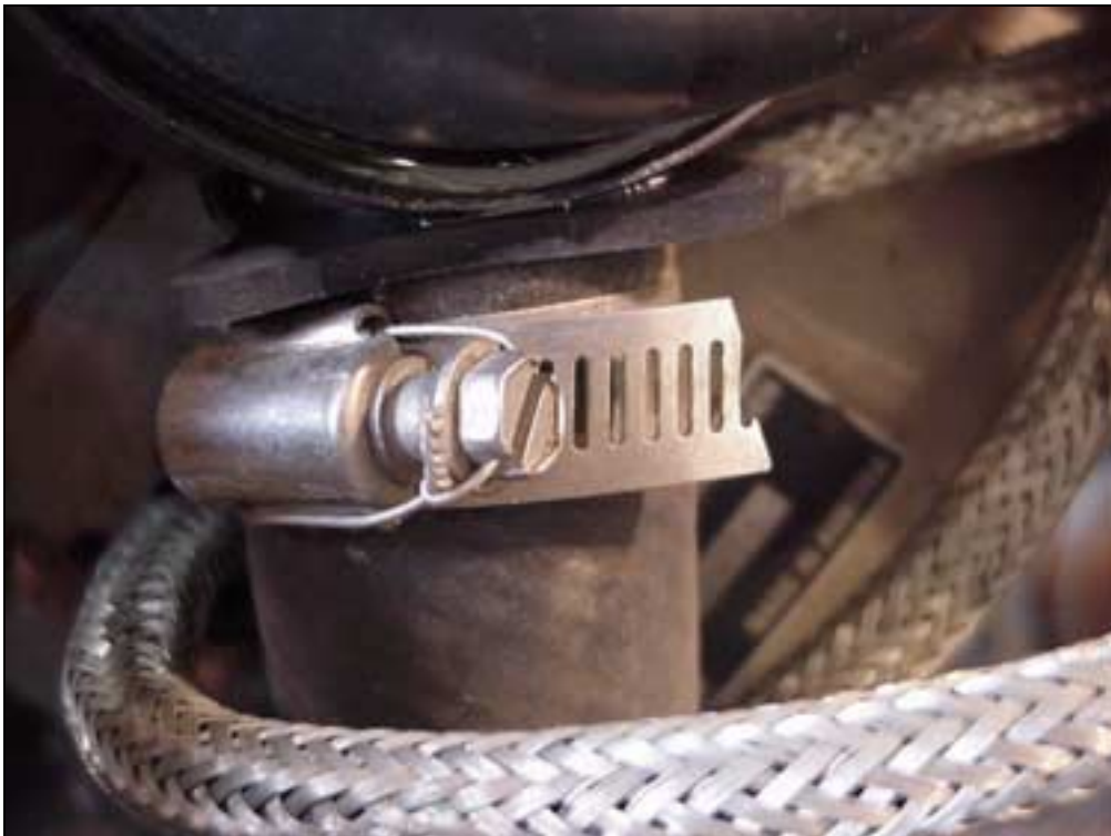
Safety wire hose clamp through the slot
