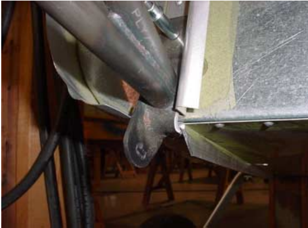
Bottom right engine mount attachment points to the firewall Check: That the Lower Bracket is not sitting on top of any rivets. 2 BOLTS AN3-5A Bolted through Firewall Stiffeners 7F7-5
