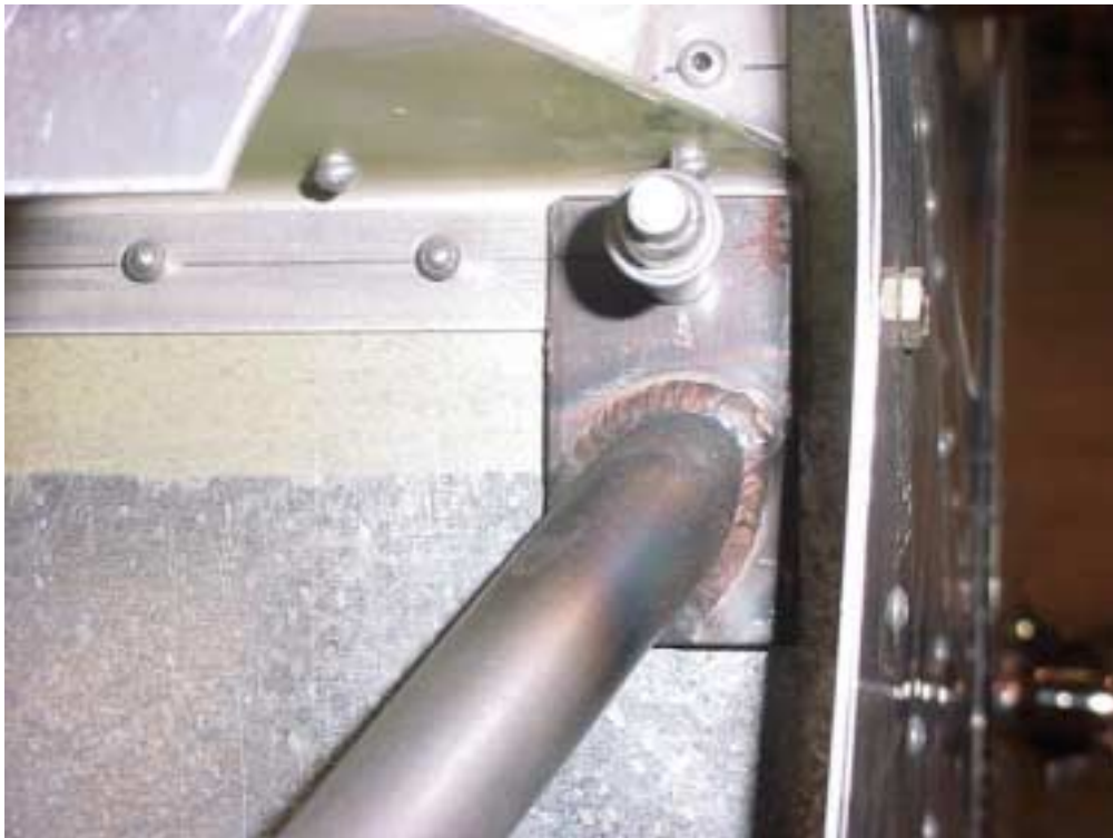
Middle firewall attachment: Engine mount plate overlaps on top of the Upper Channel 7F7-1SP. Add a .063" shim underneath the engine mount plate below the Channel (not shown).
