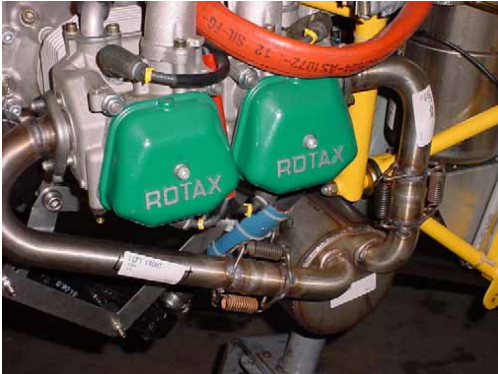
Install nuts for elbows with Anti-Seize.
