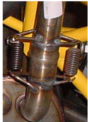
DETAIL: Spring holding the ball joint together on rear elbow.
