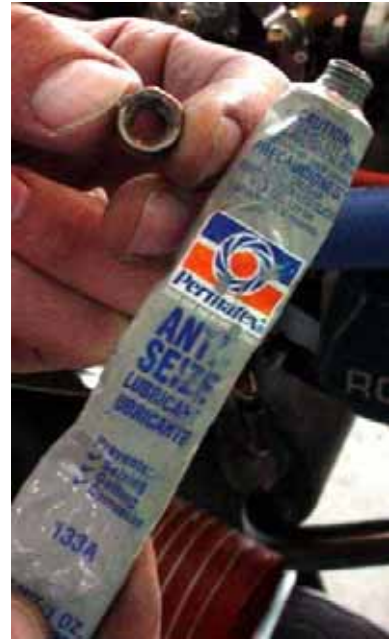
Install nuts for elbows with Anti-Seize.
