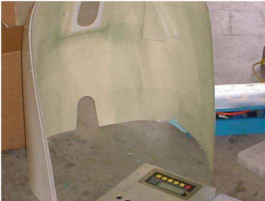
Trial fit of bottom cowl. Cutout for nose gear leg.
