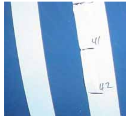
Mark off intervals of 20mm on the tape line.
