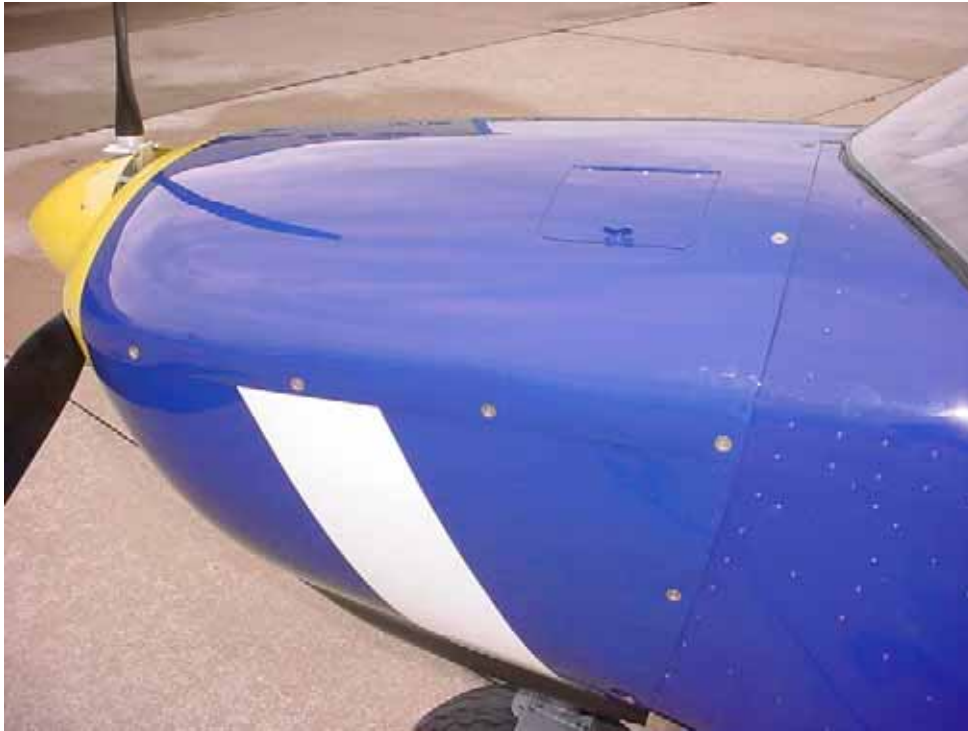
Left side view on installed cowling.
