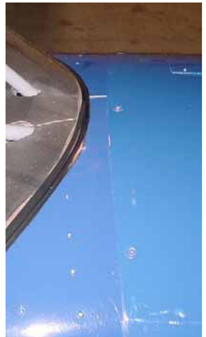
The cowl overlap on top of the fuselage skins that overhang past the firewall.
