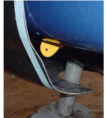
Cutout in the bottom cowl to make room for the nose gear leg.
