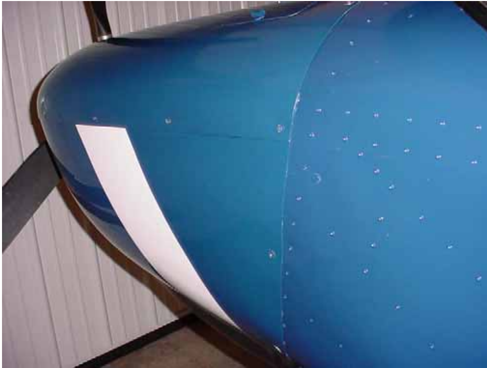
Top cowl overlaps on top of the bottom cowl. Left side.
