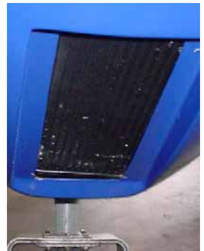
With the cowl pushed up against the radiator, tape the cowl to the fuselage and to the spinner.
