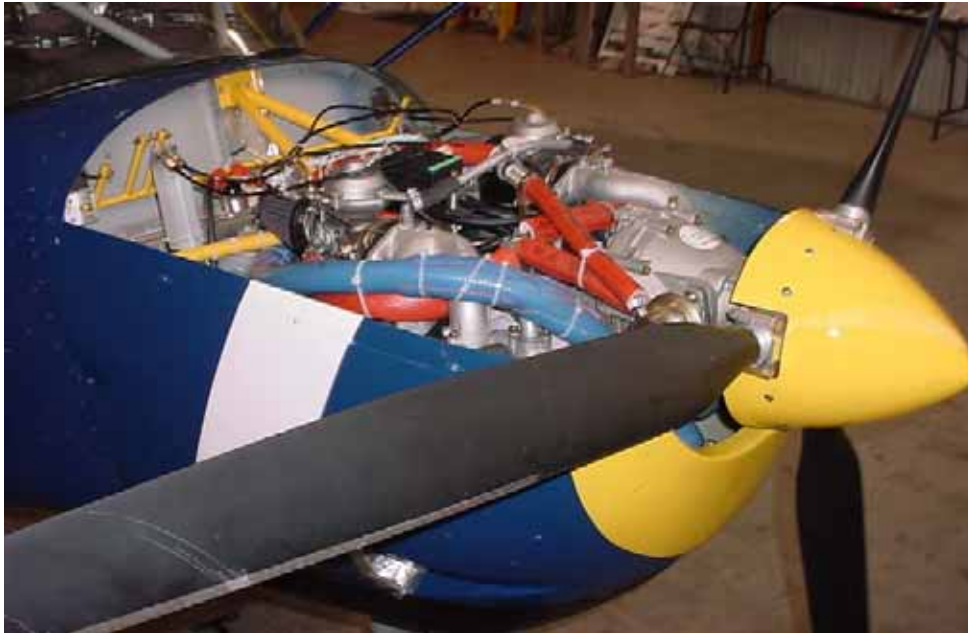
Fit cowl with the prop and spinner installed on the engine.
