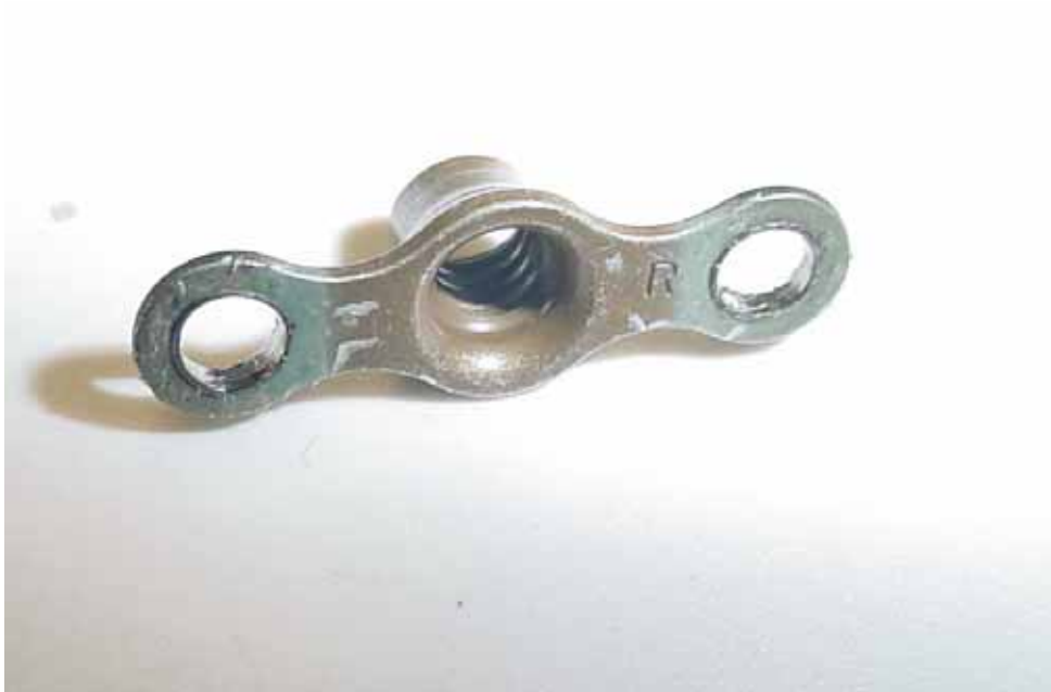
Expand the rivet holes in the nutplates with a #30 drill.
