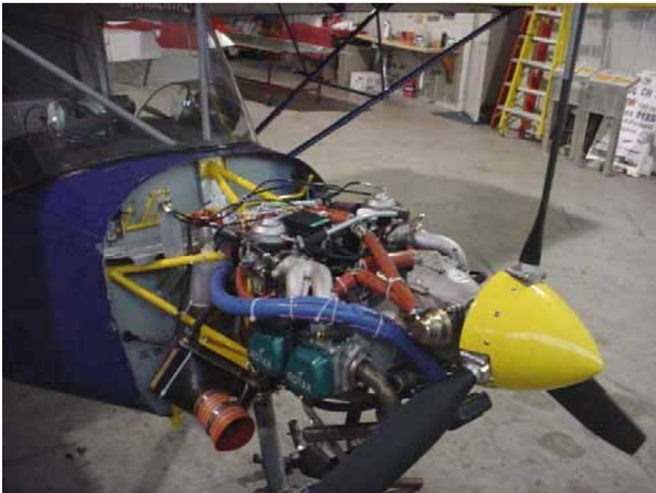
Install spinner with 9 screws.
