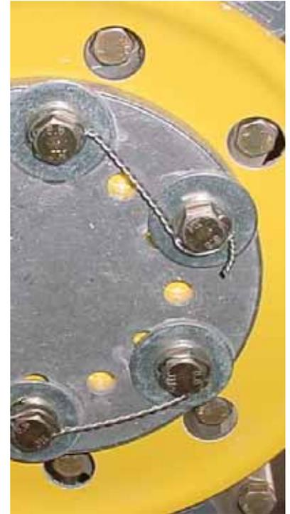
**Note:** safety wire the propeller bolts.
