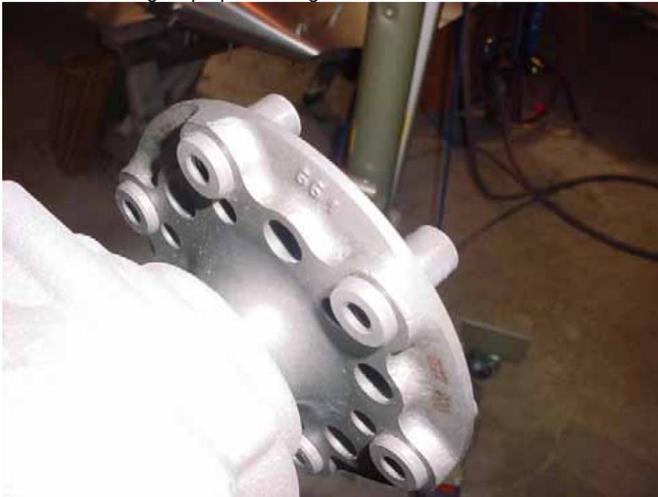
Rear view of engine propeller flange.
