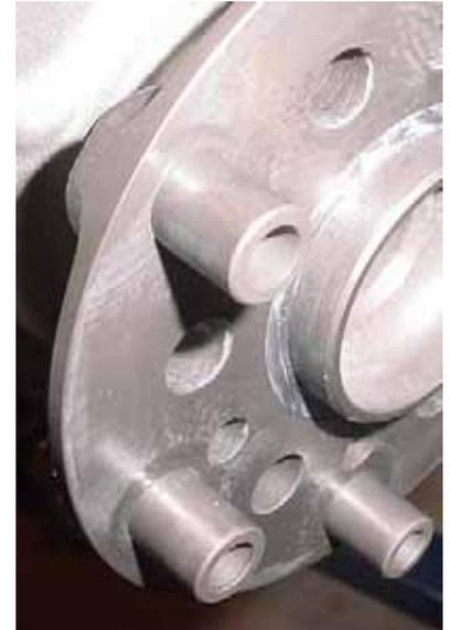
**Detail:** Front view of pressed threaded fitting.
