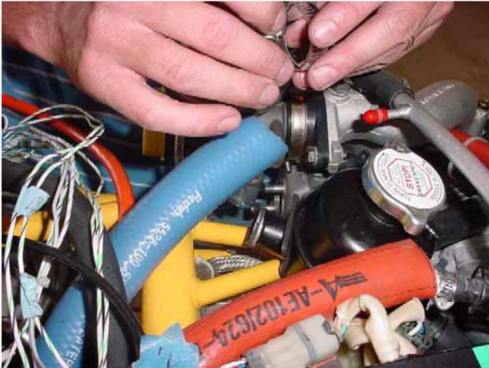
Install the hose clamp on the hose before connecting to the pressure reservoir.
