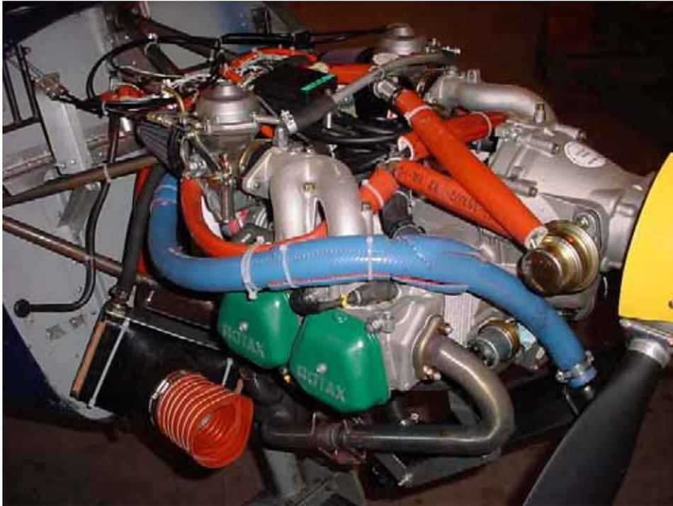
Radiator hose on the right side of the engine runs from the top of the radiator to the pressure reservoir on top of the engine.
