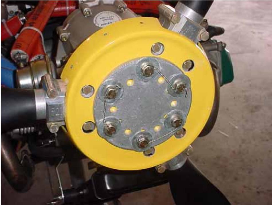
Install propeller to the engine propeller flange.
