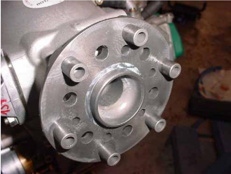
Front view of engine propeller flange.
