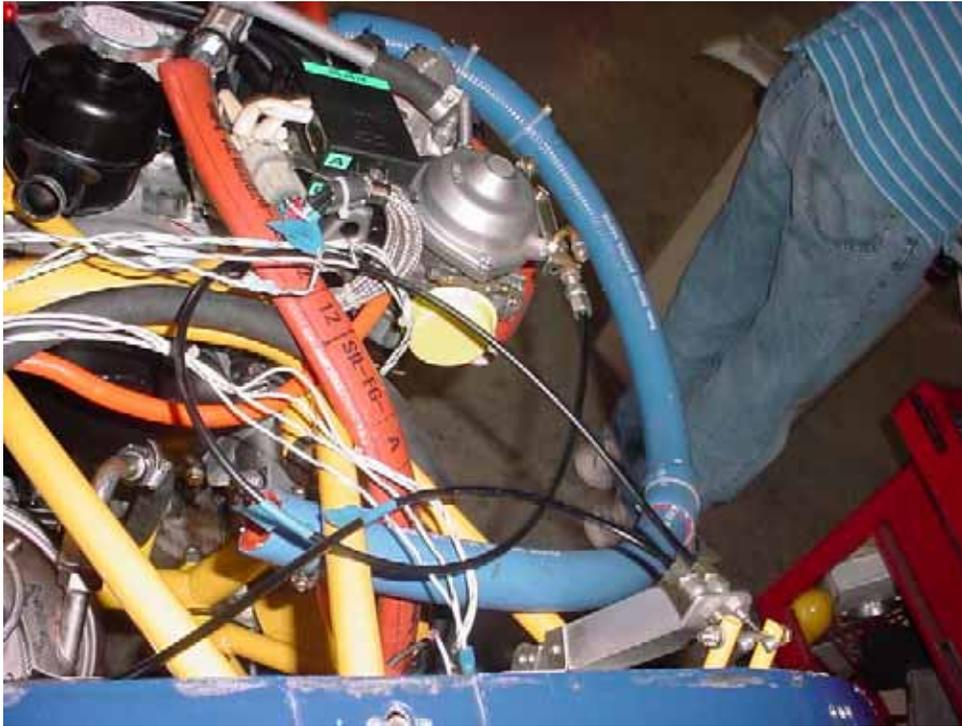
Route the radiator hose underneath the right side of the engine mount.
