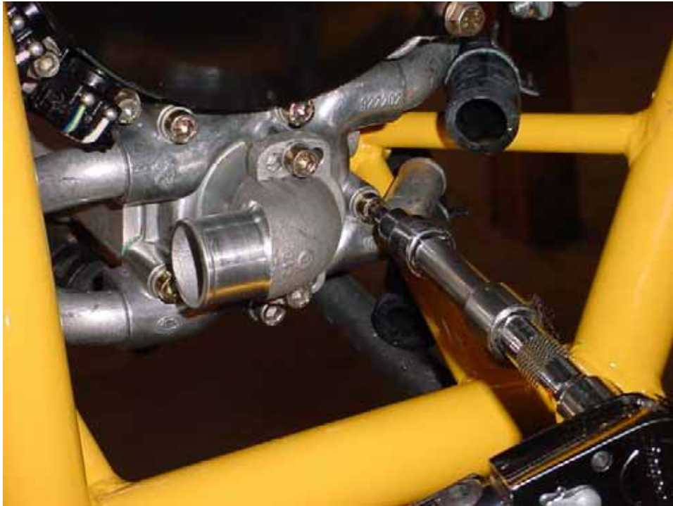
Reinstall the water pump.
