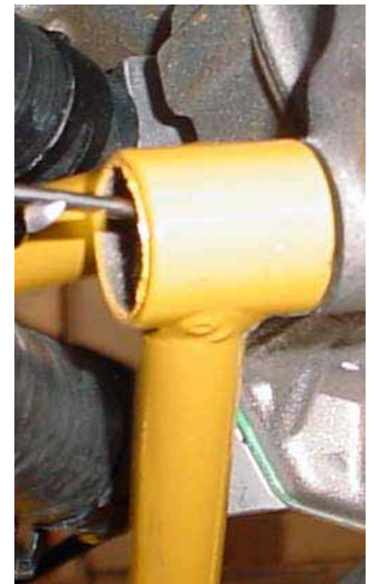
With a screw driver line up the washer.
