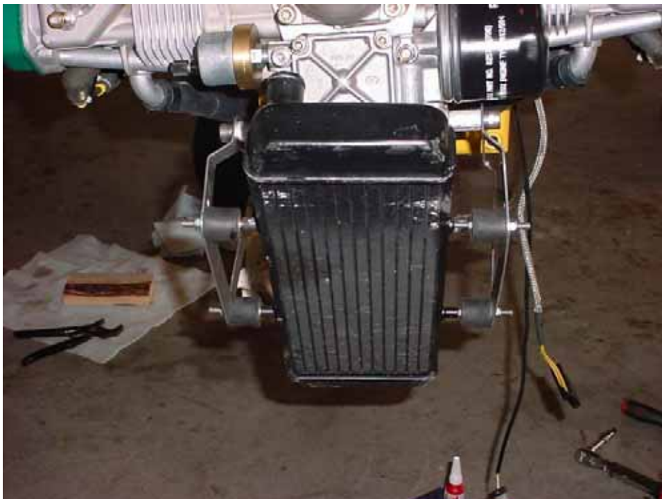
Front view of radiator on brackets.
