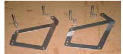
Radiator mounting brackets 1L + 1R required.
