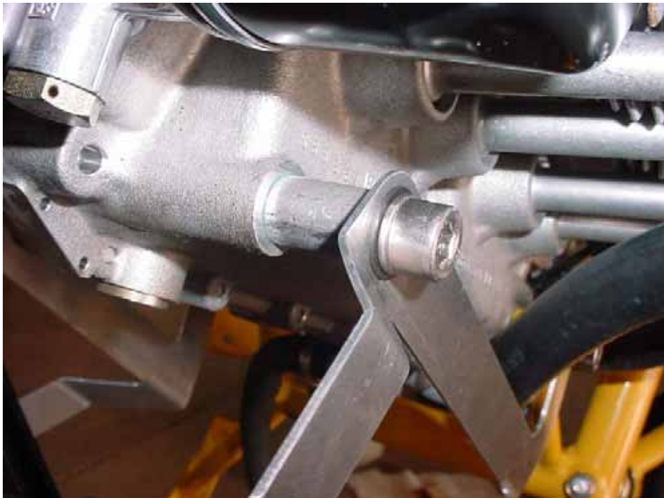
Bolt 55 with flat washer and lock washer.
