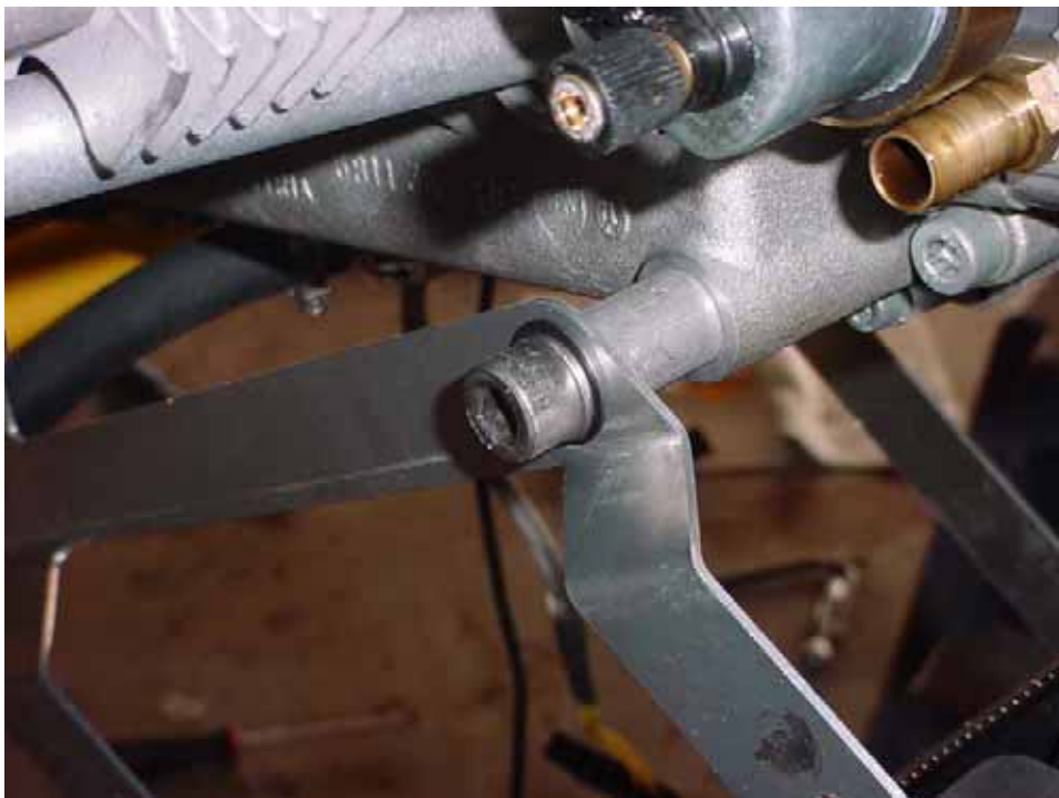
Front right bolt. Bolt 55 with flat washer and lock washer.
