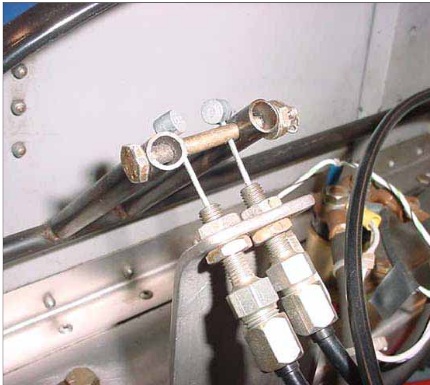
Insert the end of the throttle through the 1/16" hole in the AN3 bolt.
