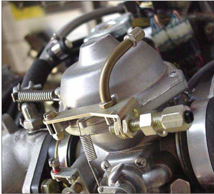
Bing carburetor, left side (throttle lever arm not in photo).
