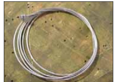
Throttle cable with formed end.
