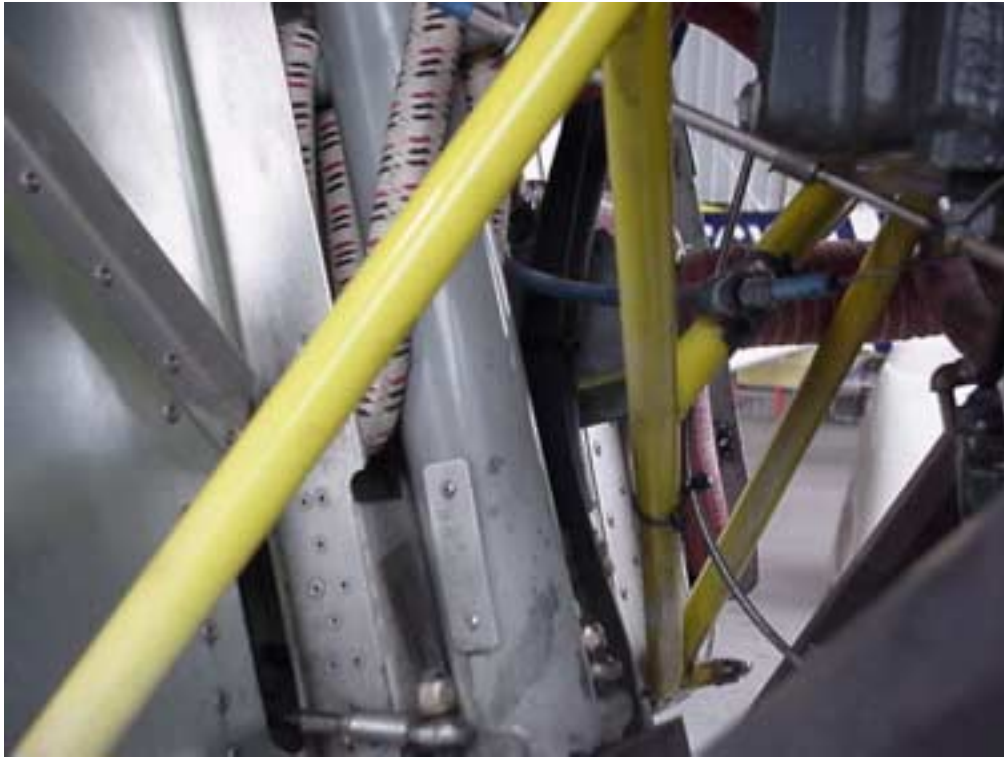
Cable on the inside of the cross tube on the left side of the engine mount
