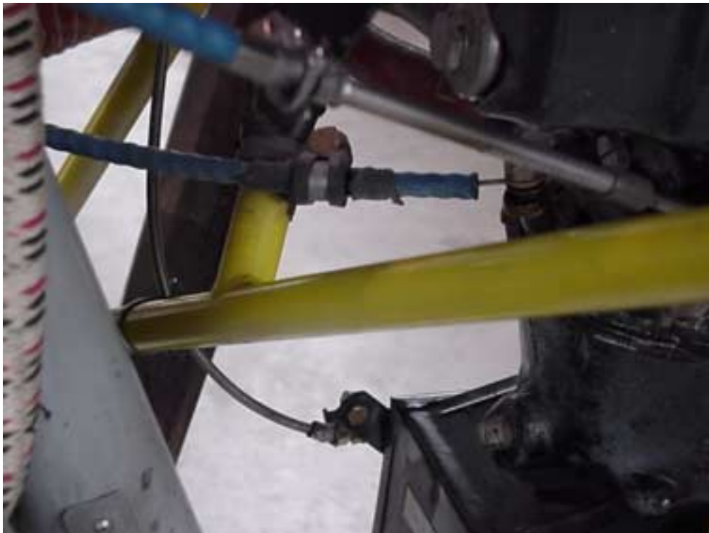
Double clamps on cable housing
