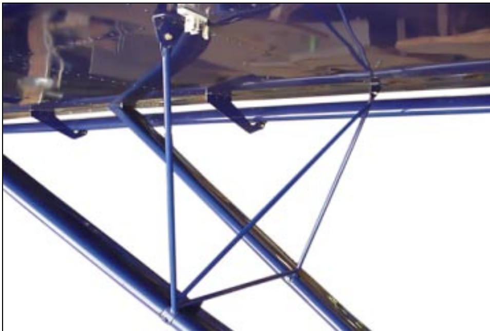
The jury strut assembly (right wing).
