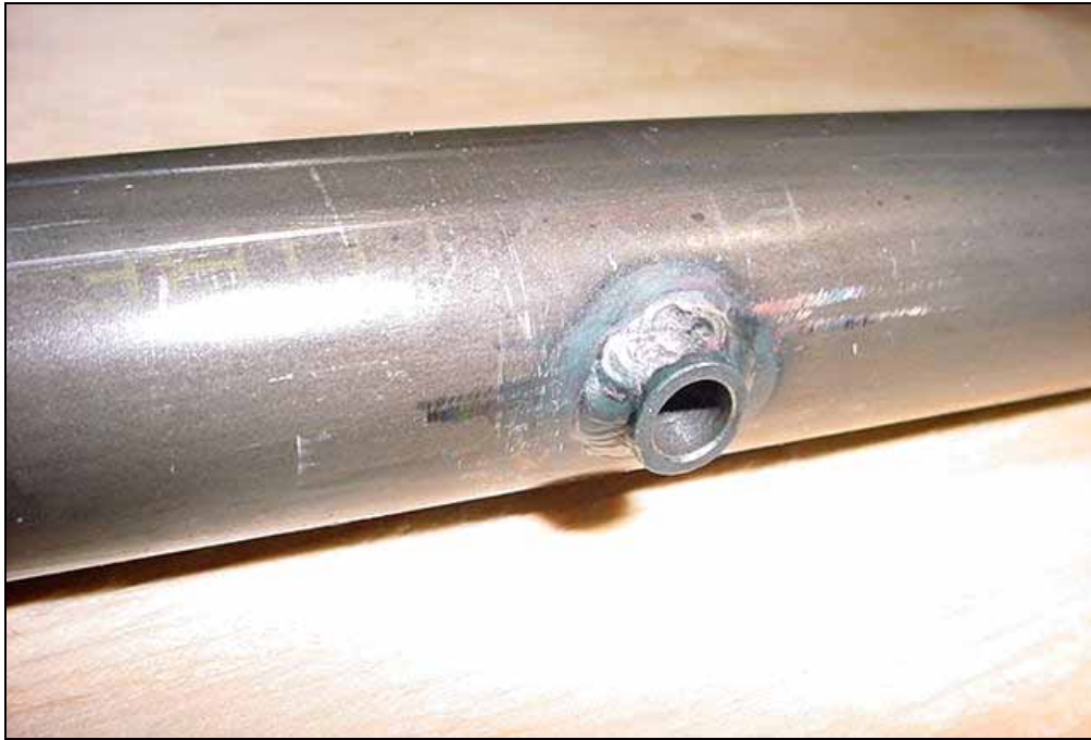
Detail of the 3/8" OD tube welded on the torque tube 6DS1-5
