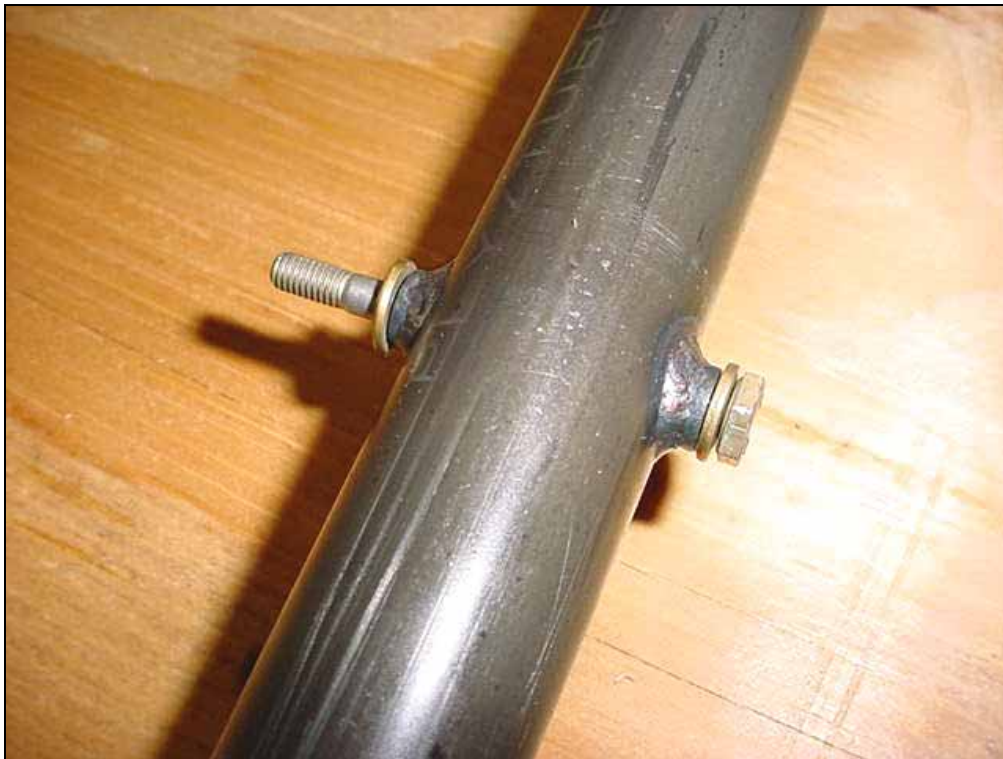
Photo does not show the Horn, remember to add the Horn 6DS1-3 under the head of the AN3 bolt.
