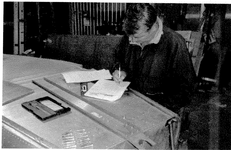
Confirming airframe material thicknesses and inspecting general condition of airframe after test
