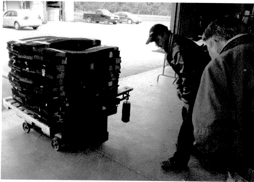
Weighing total weight of Port wing for Ultimate. Total weight is 1,148 kg
