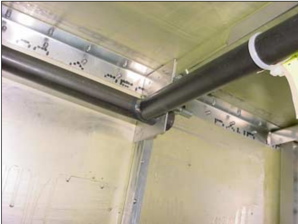
Photo of right side. Position the Flaperon Control Bearing 7F6-3 at the ends of the Flaperon Control Mount 7C3-1, then cleco the assembly inside the Fuselage.
