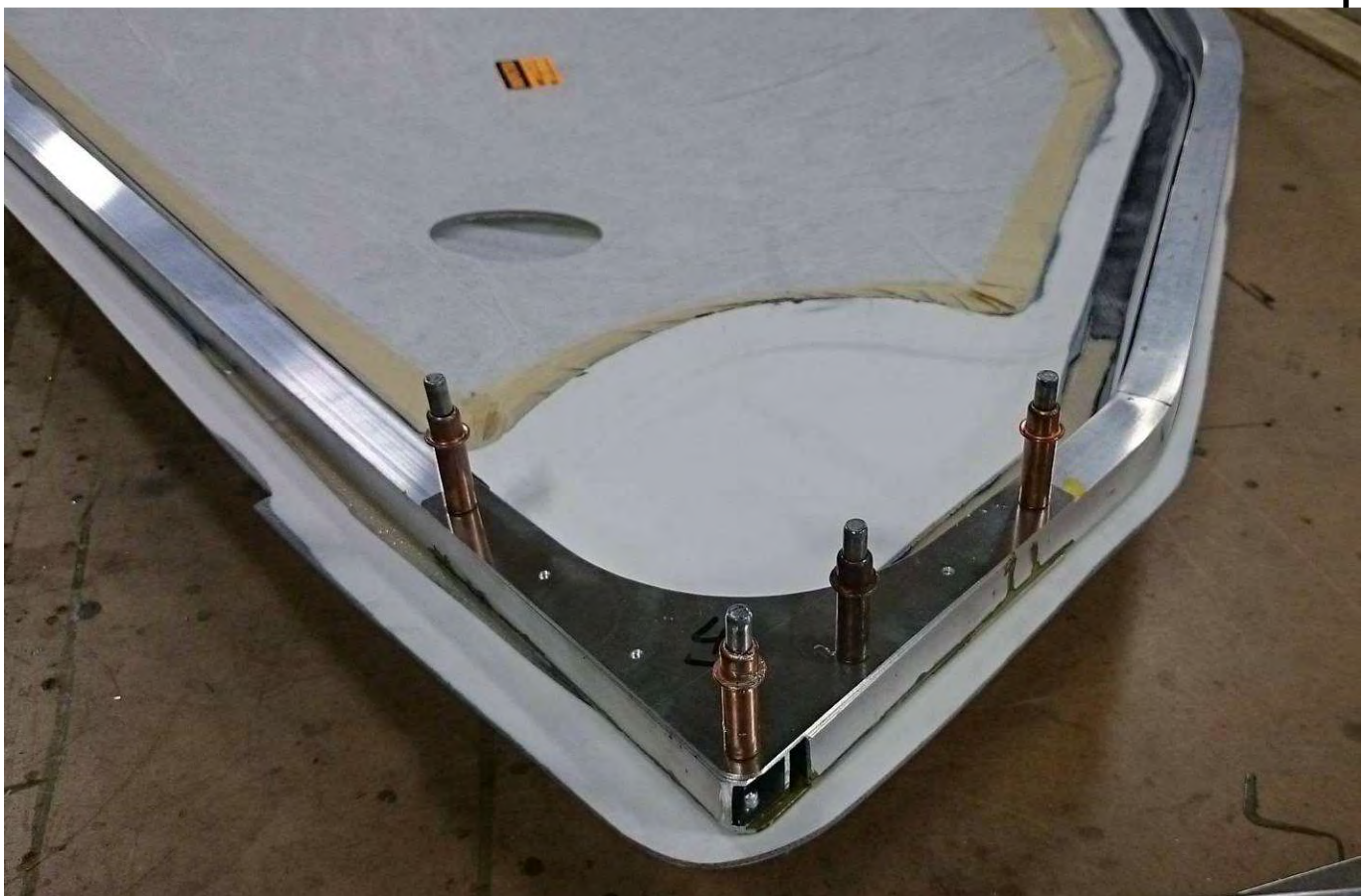
Fiberglass bubble on the aluminum door frame.
