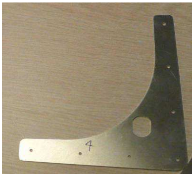
Installed on I/B gusset C75N1-9A
