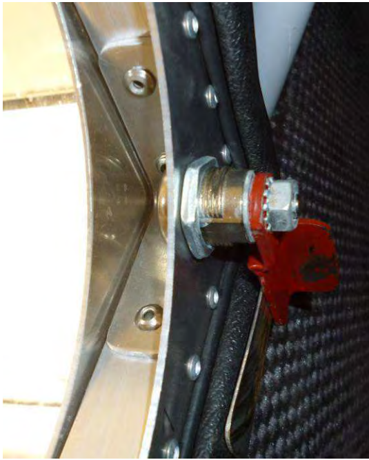
Use Loctite on the threads.
