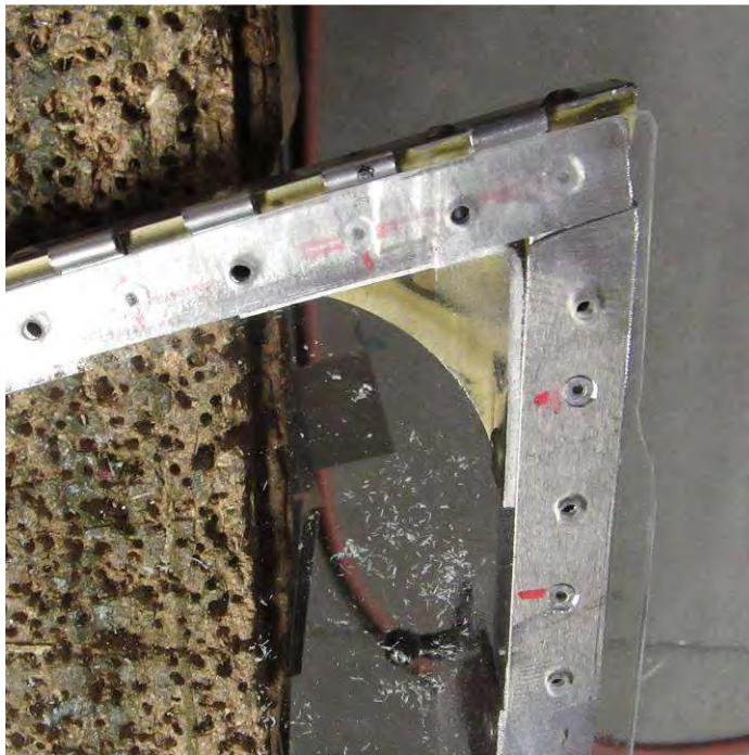
Cut the top rear edge of the bubble to make room for the rear wing attachment.. 2mm to the square tube, down 60mm
