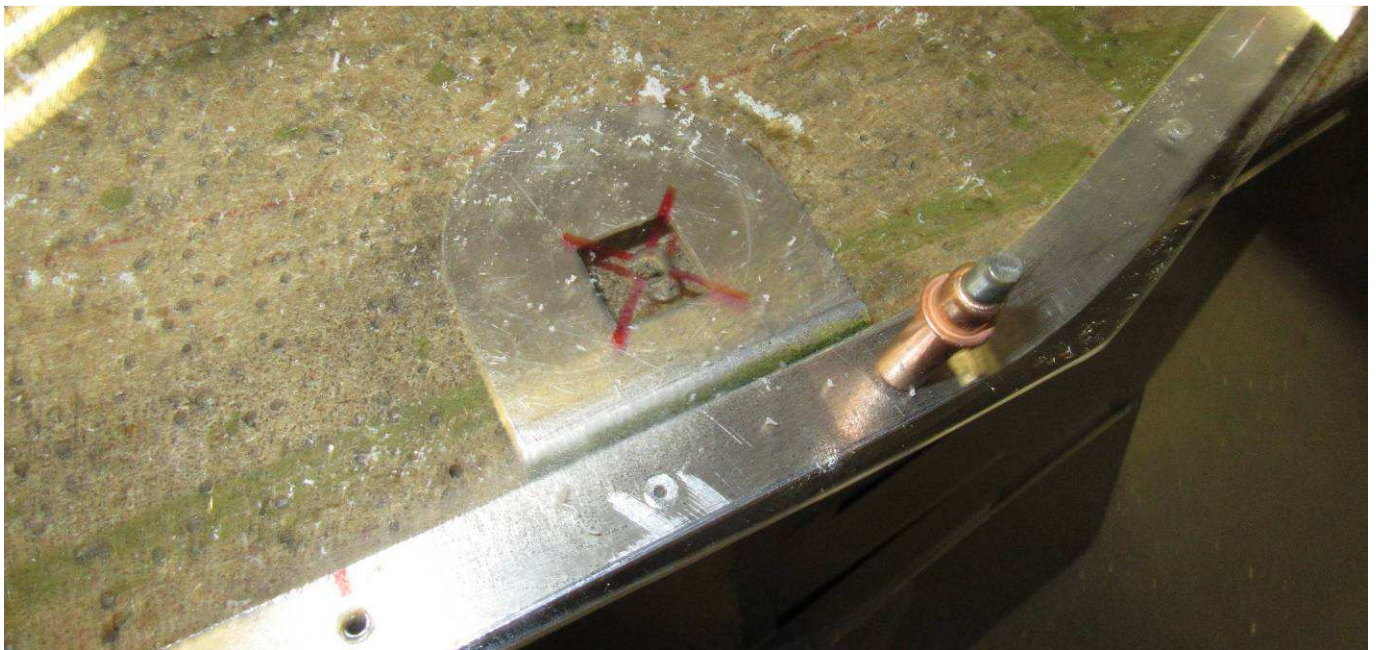
Mark the center of the square hole, drill a #40 pilot hole.
