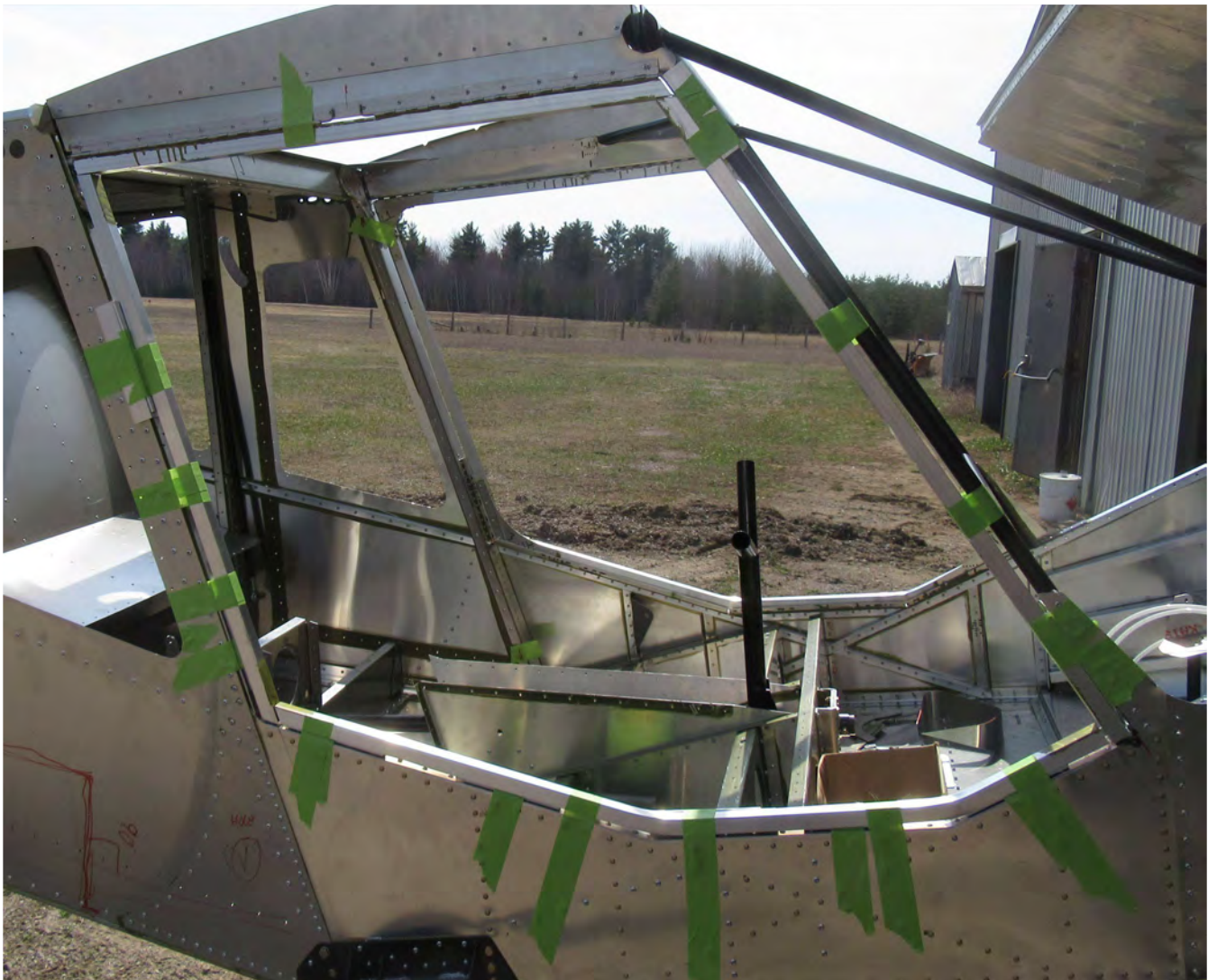
Cut the front and rear tubes to fit below the top tube. Use tape to hold the tubes on top of the spacers.
