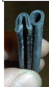
Contact of the rubber trim with the inside gusset.
