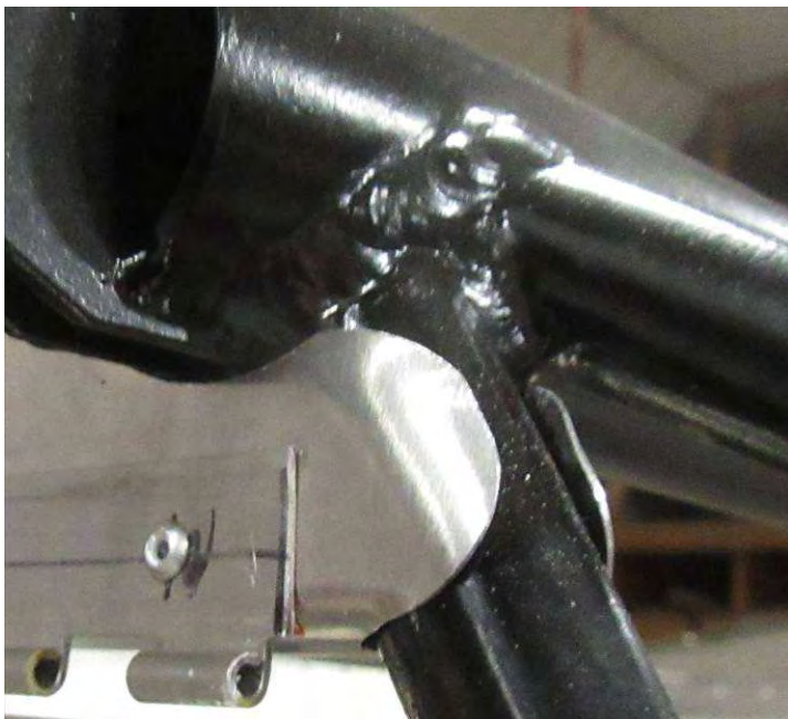
Bend the front around the tube. Add the inside rivet.
