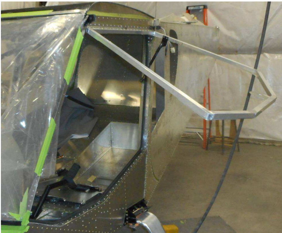
Contact of the rubber trim with the inside gusset.
