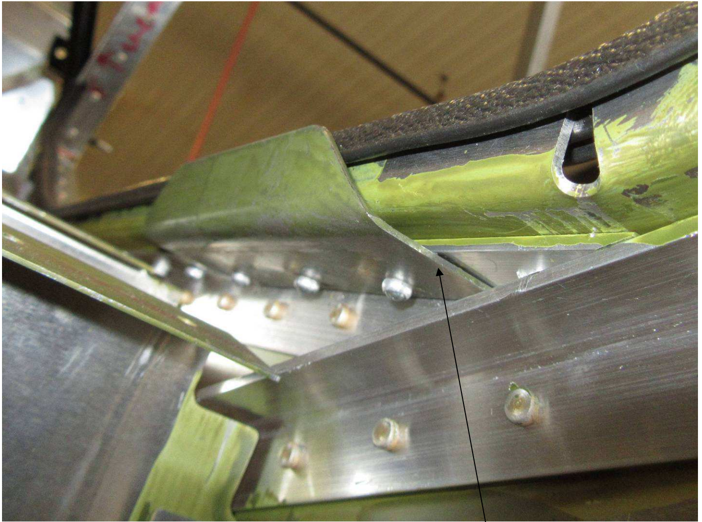
Stricker plate for the main latch: overlaps underneath the cabin side extrusion.
