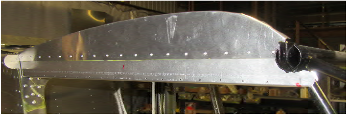
TOP WINDOW RIB C75F17-6 , riveted with A4 pitch 40 (both sides)
