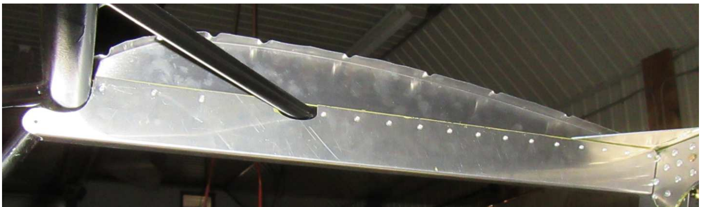
TOP WINDOW RIB C75F17-6 , riveted with A4 pitch 40 (both sides)
