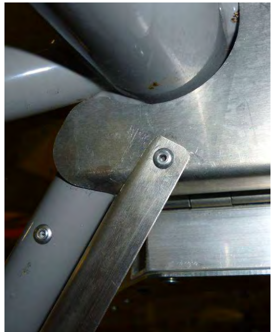
Photo showing side trim riveted to the Door Sill.
