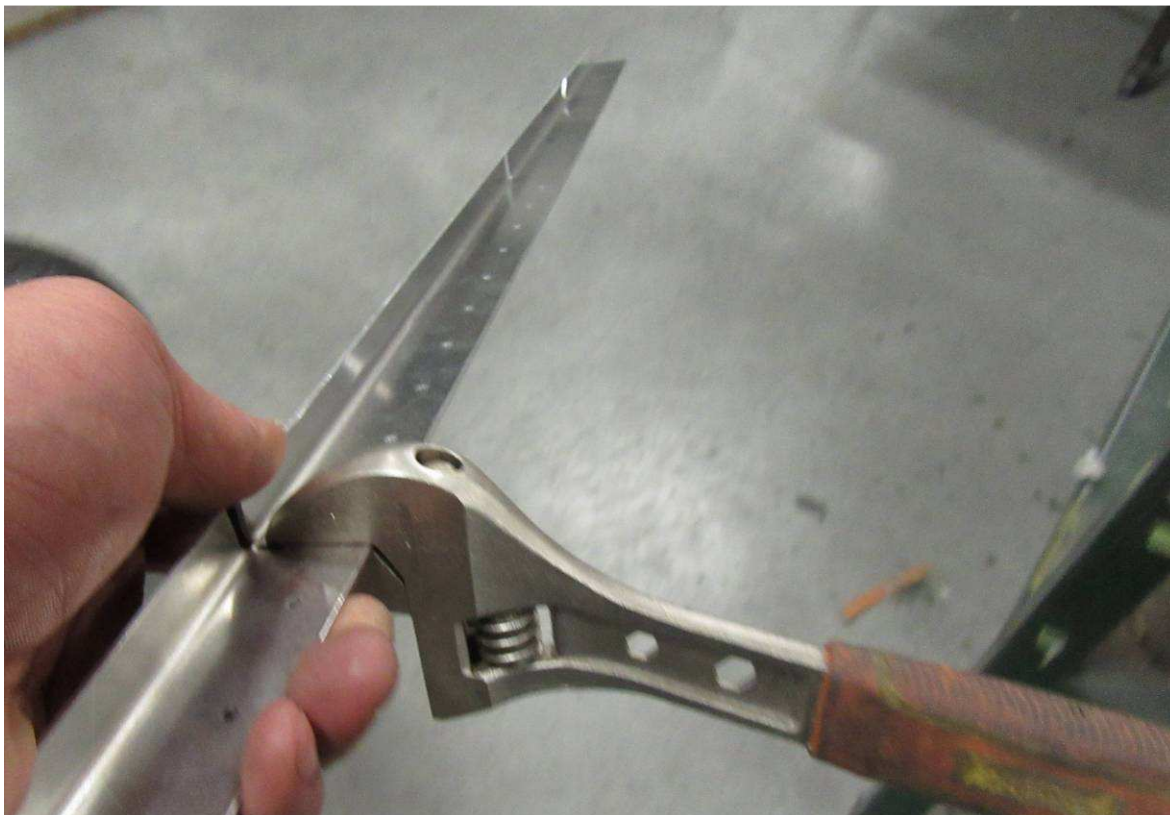
Start with the middle bends, then the front – position the Crescent wrench on the bend line and rotate the wrench to bend the angle.
