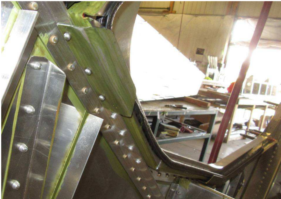
Stricker plate for the main latch: overlaps underneath the cabin side extrusion.
