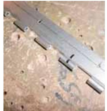
Cut the hinge section that rivet on the door to fit between the cabin frame at the front and the edge of the fuselage side skin at the rear.
