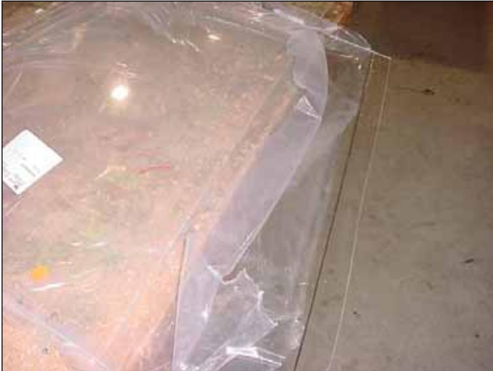
Reference line along the front edge of the extrusion. The line is approximately 12mm forward of the optic distortion line.
