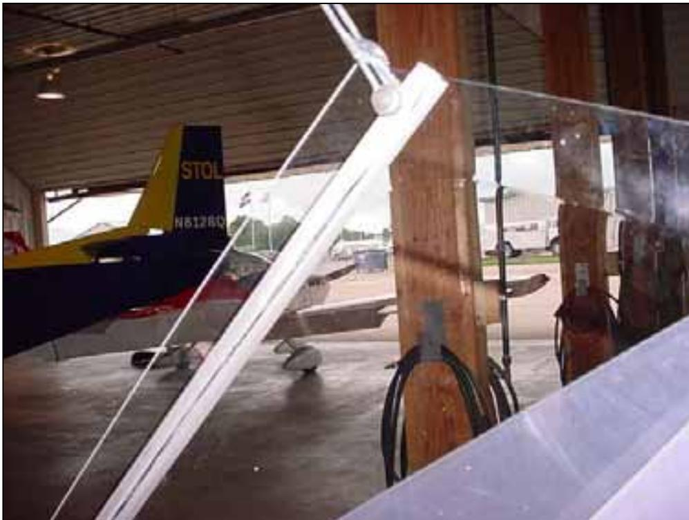
CHECK: the optic distortion line is covered by the extrusion. Hold the door upright to check that the extrusion will cover up the distortion. If necessary readjust the position of the extrusion.
