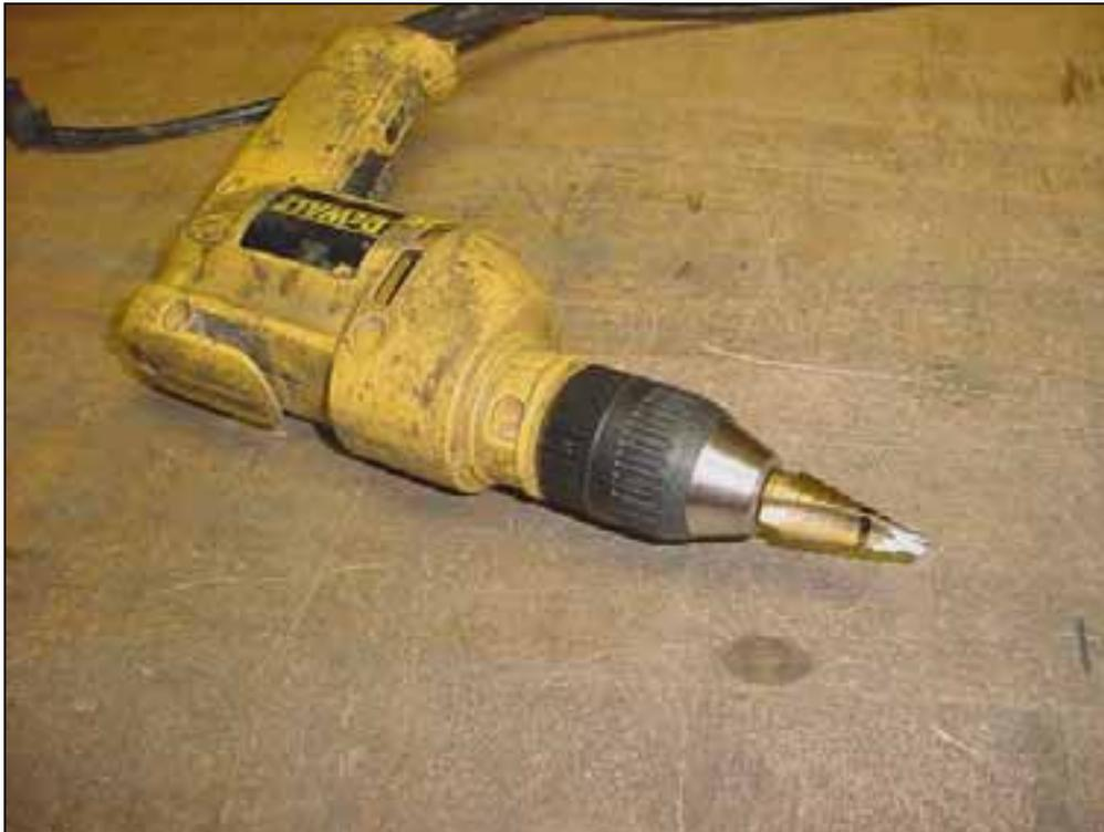
Drill half the hole from one side then finish drilling from the other side.
