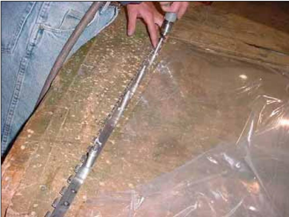
Back drill through the pre-drilled holes in the hinge to Cleco the hinge to the bubble door.
