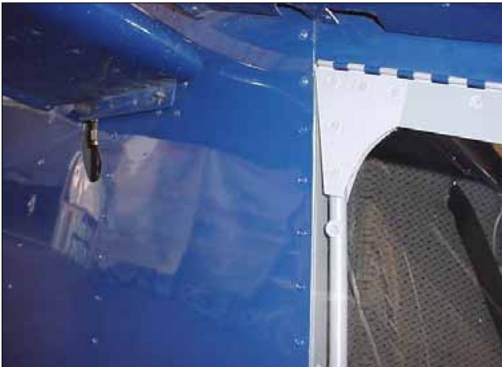
With the hinge in place, position the bubble door on the fuselage, the reference line is behind the windshield trim, the top edge is just below the spine of the piano hinge.
