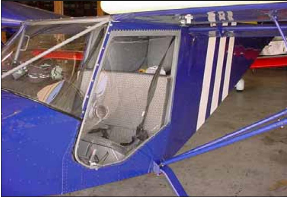
The front of the bubble door is trimmed back to fit behind the Side Windshield Trim 7F19-8M. An aluminum extrusion is installed over the front edge of the door parallel to the side tube of the cabin frame. Plan to leave approximately 2mm gap between the front edge of the extrusion on the door and the back edge of the trim.
