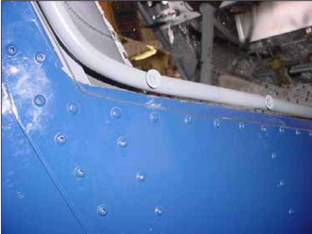
CHECK: The door is height as possible on the fuselage, the bottom edge of the bubble door overlaps the cabin frame.
