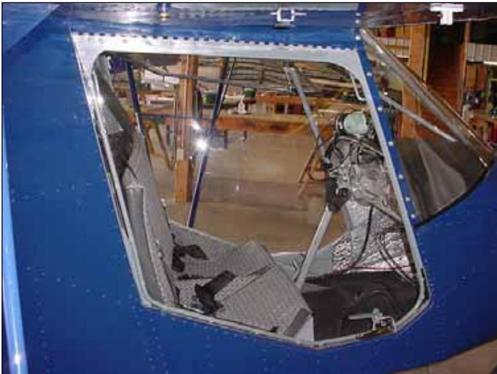
Keep the door as height as possible and still have approximately 8mm overlap long the bottom with the cabin side.
