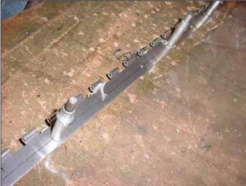
Position the bubble door flat on the workbench, lay the hinge on top of the bubble door. Line up the hinge with the previously made reference line when the door was on the fuselage.
