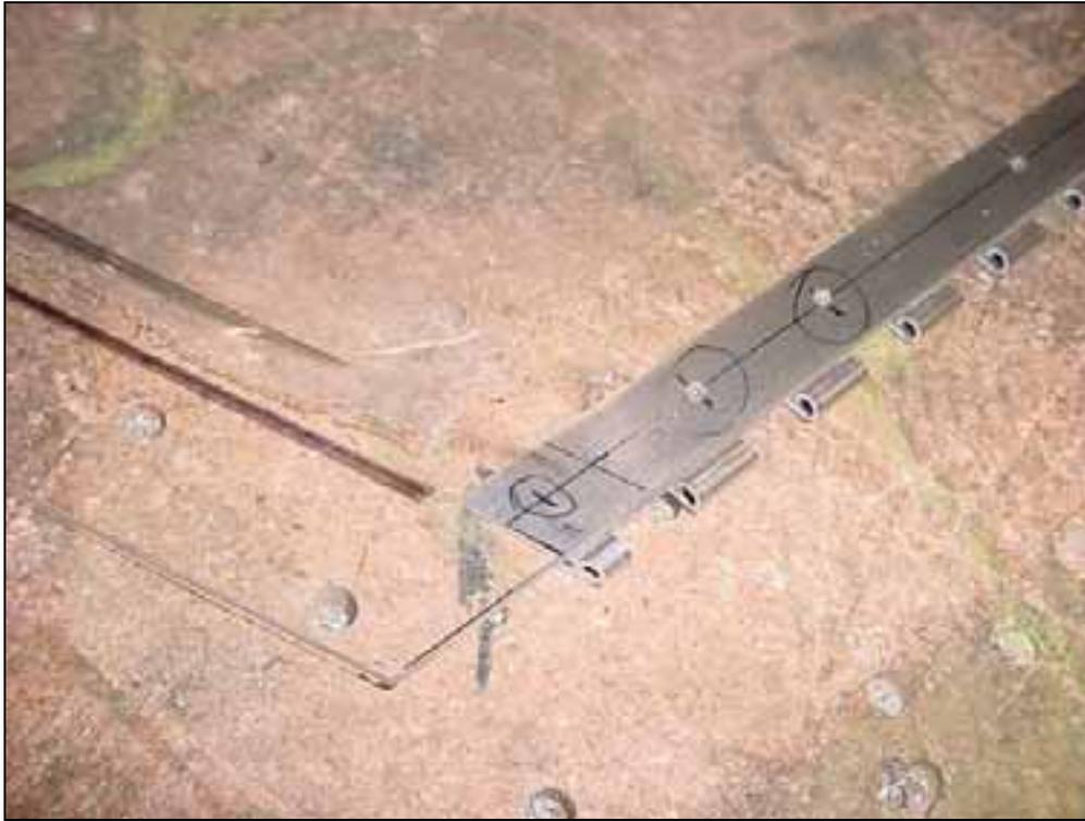
Each leg of the top Gusset is 70mm, Ref middle diagram on drawing 7-F-19 (Gusset at top of Bent Door Frame 7F19-2 and the Upper Tube 7F19-3)
