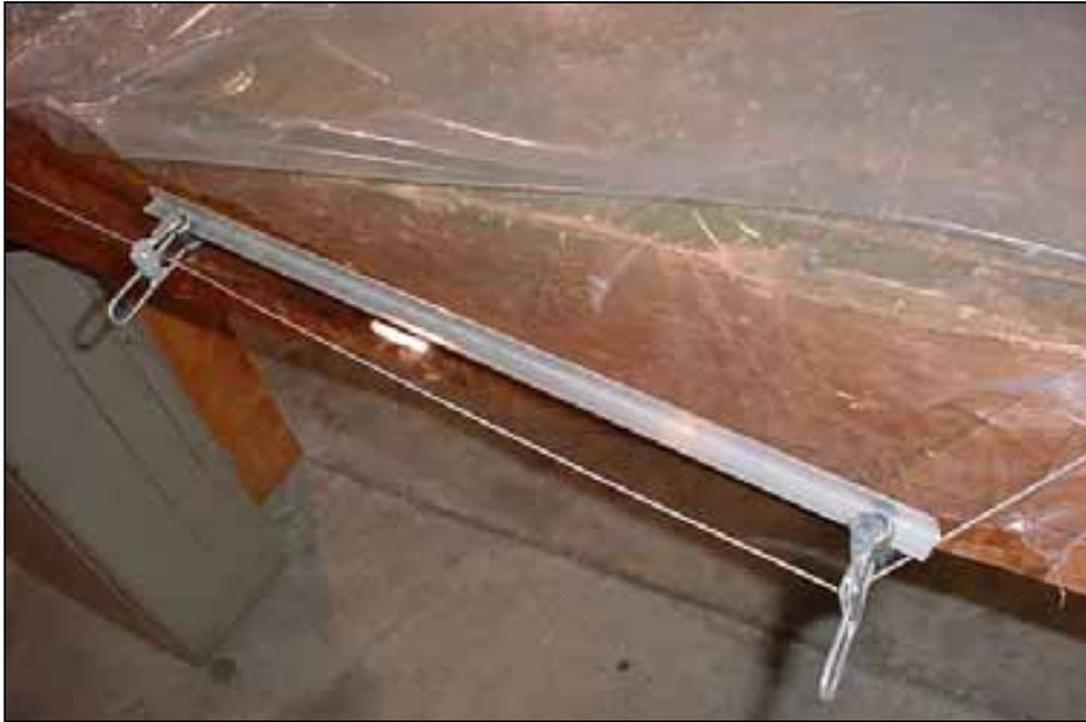
Peel back the protective plastic sheet to expose the flange on both side of the bubble door.
