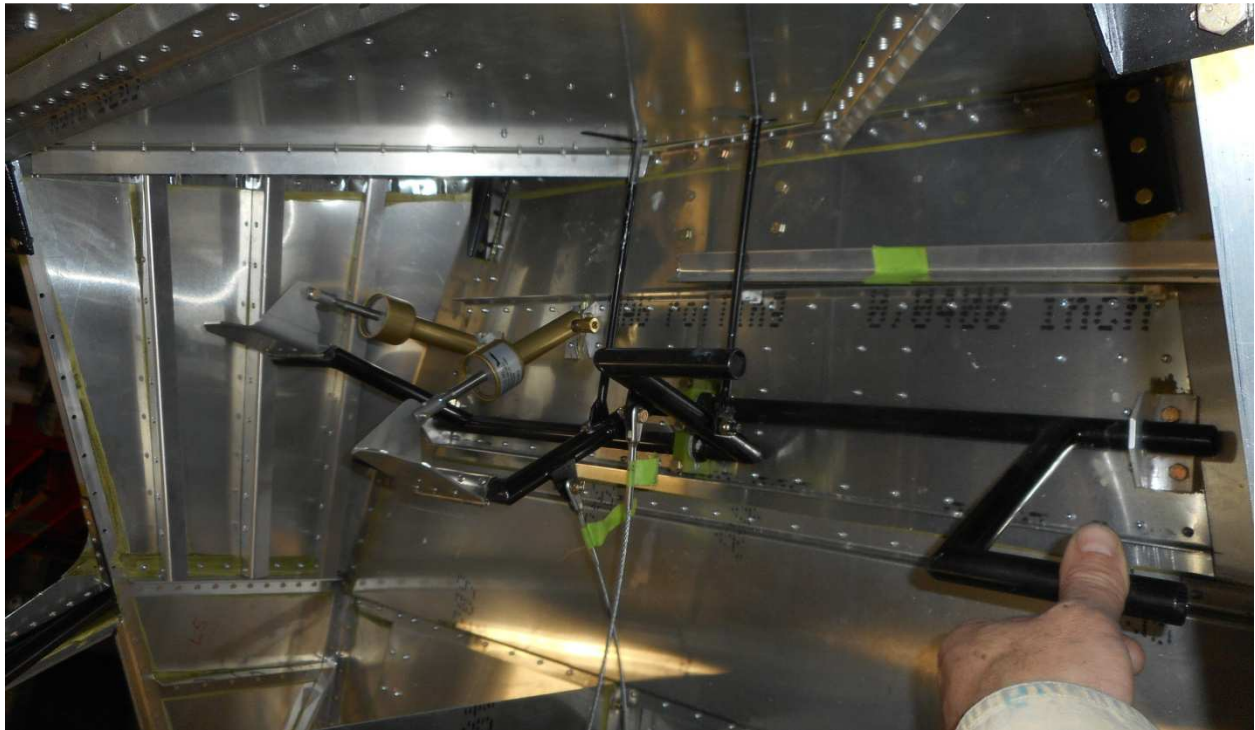
Rudder pedals deflections are limited by the rudder stops and the nose gear leg.
