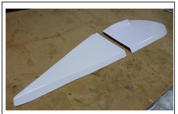
Cut the access material around the flange.
