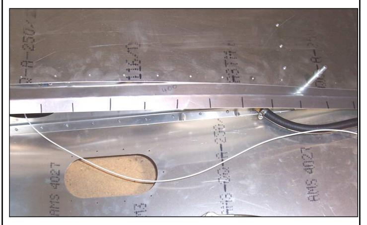
Lay the Wing Root Angle on the Wing. Place a mark between the rivet locations.
