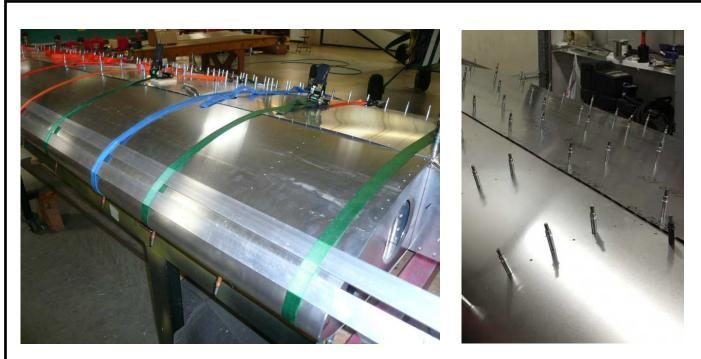
Using ratchet straps and a 1" x 2" board pull the Nose Skin around the Nose Ribs. The Nose Skin should slide under the Top Skins to be drilled. The Nose Skins will be riveted on top of the Top Skins after deburring. Be sure to place a piece of plywood under the ratchet on the strap or the metal ratchet will dent the Top Skins.
