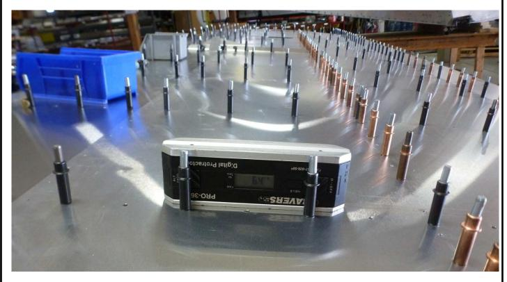
**Note:** It is a good idea to check that the Spar is still vertical before reassembling the Skins and riveting. Even after the holes are drilled there is enough play in the Clecos to introduce twist if the Spar isn't vertical.
