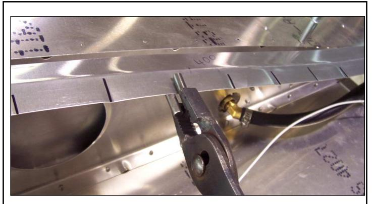
Put crimps on the marks in the flange of the Wing Root Angle to match the curvature of the Ribs.
