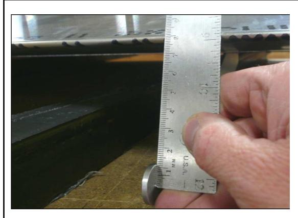
Set the Trailing Edge Skin height at 80mm from the hole in the Flaperon Arm to the center of the radius of the Trail Edge Skins.
