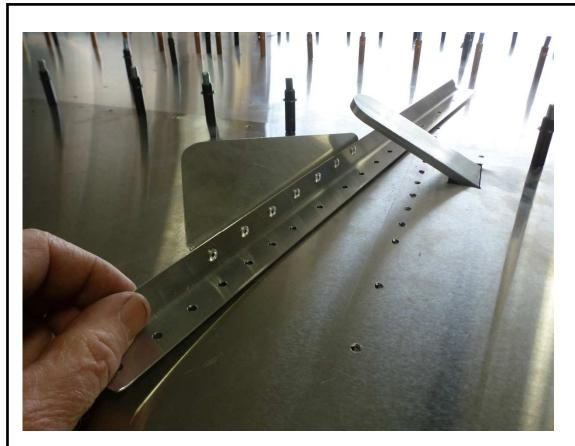
Rivet the strut fitting doubler to the strut angle.
