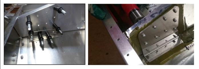
Position the L angle against the Bottom Skin and the Flaperon Arm. Back drill through the Flaperon Arm into the L angle and cleco. Then back drill the holes in the Bottom Skin into the L Angle. Expand the holes with a #30 drill bit. Remove the Flaperon Arm and L angle from the Rear Rib, deburr the holes.
