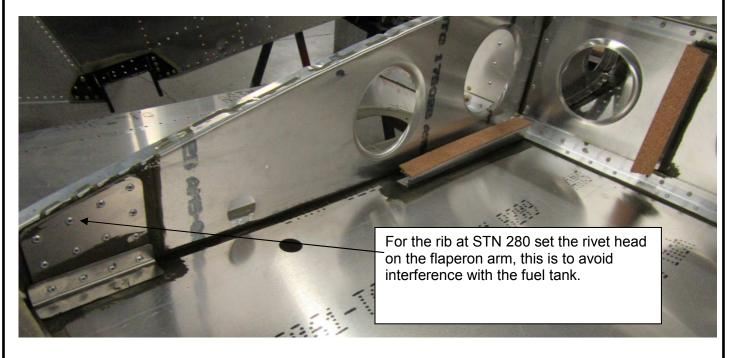
Rivet the Flaperon Arm and L angle to the Rear Rib with A5
