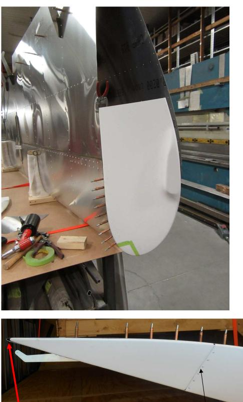
Fit the Nose wing tip inside the leading edge and clamp in place. When the part fits nicely, drill and cleco.
