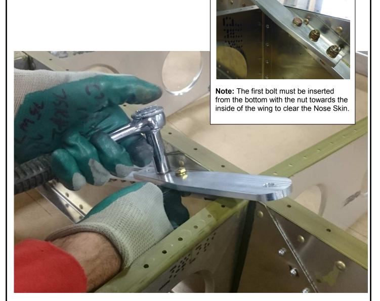
Bolt the Front Upper Strut Fitting to the Strut Angle on the Spar with 3 AN4 bolts.
