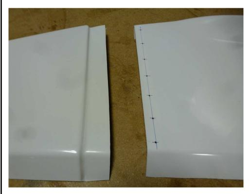
Pre-drill the holes in the Nose wing tip only.
