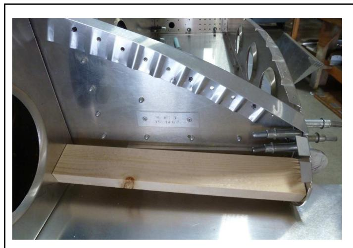
Cut a board to act as a support for the root nose rib.
