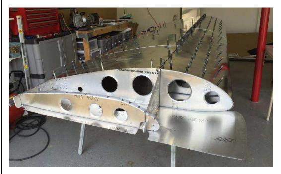
With the I/B Nose Skin strapped tight to the Nose Ribs, back drill, with a #40 drill bit, the holes into the Nose Ribs and Spar. Cleco every hole in the Nose Ribs and every other hole in the Spar.
