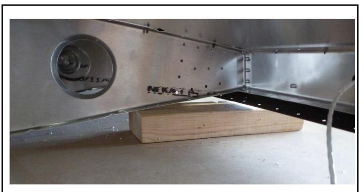
Block under the rear ribs to keep the spar vertical.
