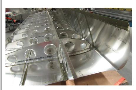
Flip the Wing over and set it on several beams. 2"x2" steel beams are used in the photo above but any rectangular or square beam 2" tall will work to lift the wing above the workbench. It is a good idea to place a piece of plywood under the Rear Channels on the beams to prevent the Wing from rocking.
