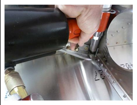
With the front upper strut fitting bolted in place, the rivets are pulled from the top side of the wing. (After the wing is turned over).
