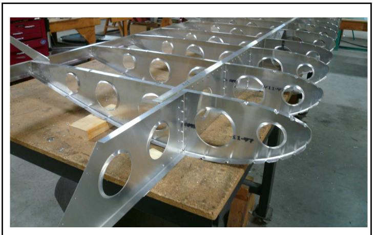
**Check:** Check that the Spar is vertical at several locations down the length of the Spar. This will prevent twist being built into the Wing.
