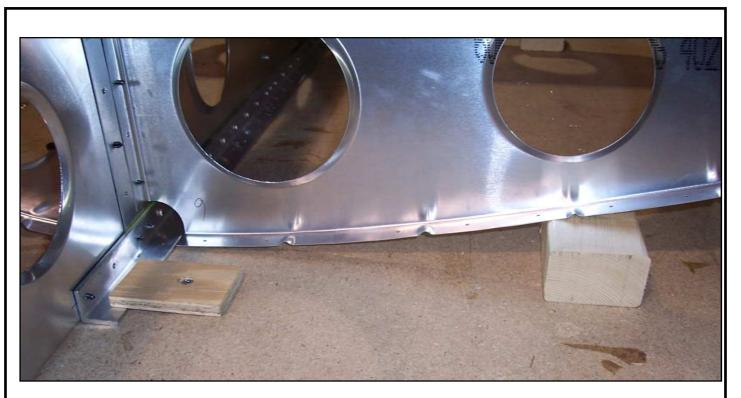
Screw pieces of plywood to the workbench to secure the Wing Skeleton. Slide pieces of 2"x4" under the Rear Ribs to rotate the Spar till it is vertical.
