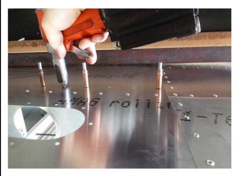
Rivet the bottom side of the wing to the spar and ribs. Also rivet the strut angle.
