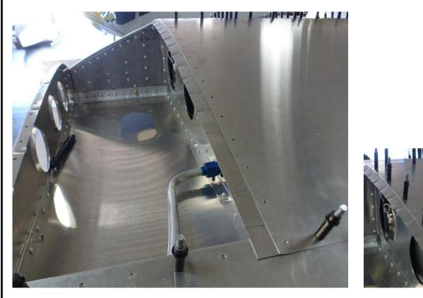
Crimp the L angle to match the angle of the Wing Root Angle and the Root Nose Rib. Be sure the Crimps are between rivets locations.
