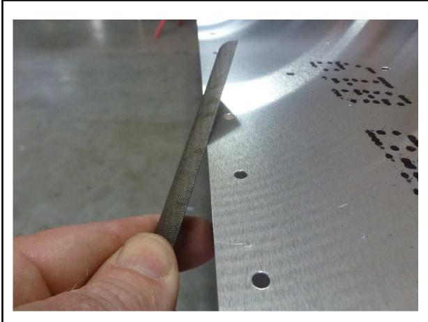
Remove the Skins from the Skeleton, deburr, reassemble.
