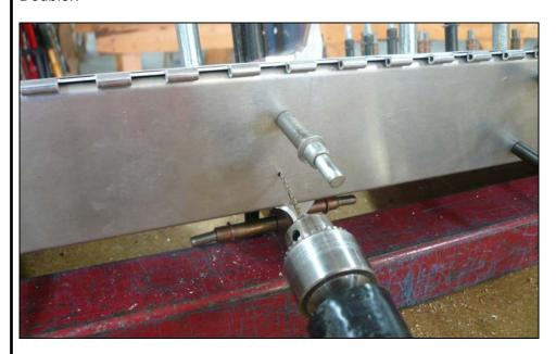
Use a #40 drill bit to back drill through the holes in the Skin into the Angle and cleco. Expand the holes to a #20 and cleco.
