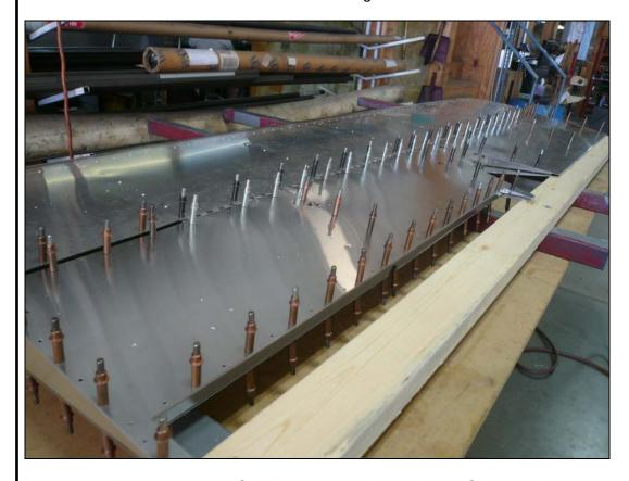
Position the Elevator onto the Stabilizer with the Piano Hinge. Slide the Piano Hinge between the top Skin and flange on the Elevator. Center the Elevator onto the Hinge that is attached to the Stabilizer. Use a #40 drill to back drill through the Skin into the Hinge. Then open up all holes on the Hinge to #30 and then final size to #20 and cleco.
