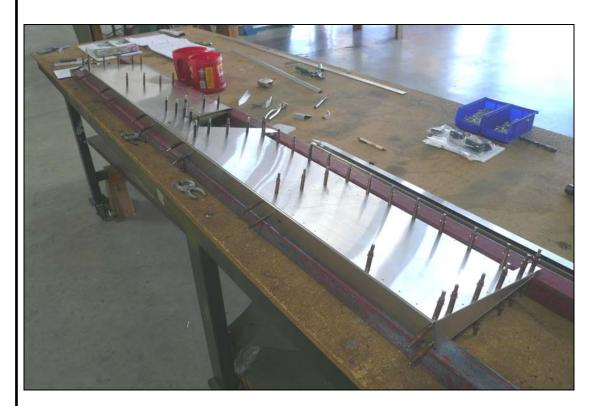
Lower the top Skin on the Elevator and cleco the Skin to the Ribs and Channels. Notice the beams keeping the Elevator off the work bench.
