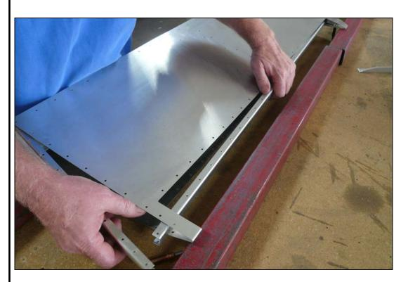
Slide the Cutout Channel into place on the Elevator. It will be helpful to pull the outboard Rib away from the Channel to slide it in place. Cleco the bottom flange of the Channel to the Skin.
