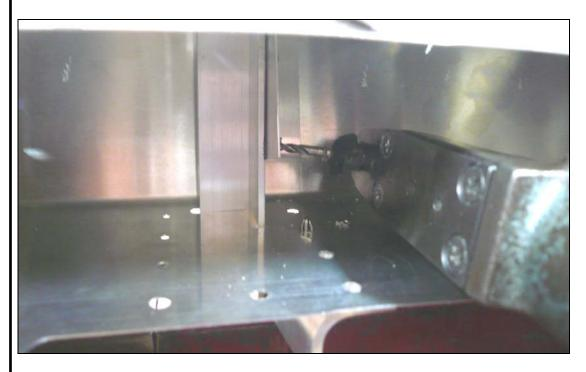
Reinstall the Angle in the Elevator. Use an Angle drill with a #30 drill bit to back drill through the Angle into the Doubler and cleco. Expand the holes with a #20 drill bit and cleco.
