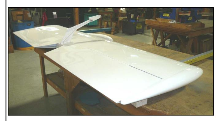
The Elevator and Stabilizer can be mounted together and painted as one unit. After the assembly has been painted the Elevator can be Mass Balanced before mounting on the Fuselage. Balancing the control section will be shown later in the Drawings and Manuals.
