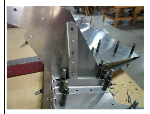
The 110mm long L Angle is installed on the top of the Elevator. Cleco the aft hole in the L Angle to the Elevator and Rear Channel. Back drill through the L Angle into the Elevator and cleco. Expand the holes with a #20 drill bit and cleco.
