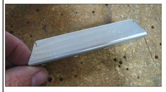
Remove the L Angles from the Elevator. Mark a point 10mm from the end of the undrilled flange. Mark a line from the point to the start of the bend radius. Crop the corners of the L Angles and cleco them on the Elevator.
