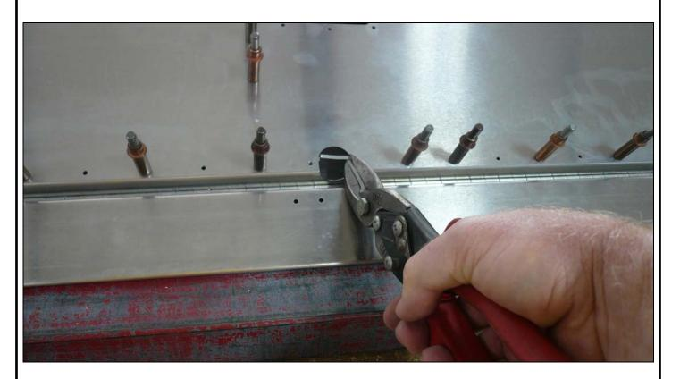
Use a pair of Snips to remove the tab on the bottom of the Trim Tab Channel. Then use a file to smooth the cut flush to the Skin.
