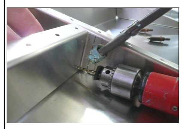
Slide the L Angle into position on the Rear Channel and Inboard Rib. Position the L Angle so the predrilled flange is on the Inboard Rib. Clamp the L Angle to the Inboard Rib and back drill through the Rear Channel into the L Angle with a #30 drill bit and cleco. Expand the holes with a #20 drill bit and cleco. Install and drill the L Angle on the opposite end of the Channel.
