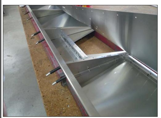
P/N: C75T3-7 Elevator Center Channel
