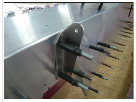
P/N: C75T4-1 Lower Elevator Horn
