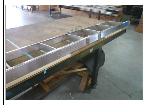
Once the Ribs and Front and Rear Spars are riveted together. Position the skeleton upside down on the work bench and secure the back Spar using plywood scrap. Level the Front and Rear Spar.
