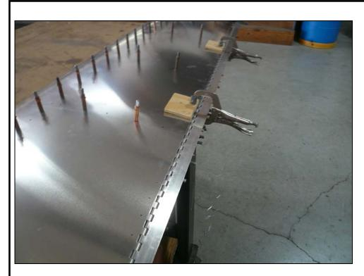
P/N: C75T2-5 Elevator Piano Hinge
