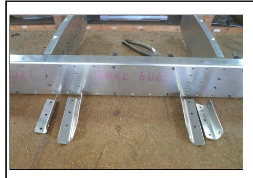
P/N: C75T2-1 Front Spar Attachment Bracket
