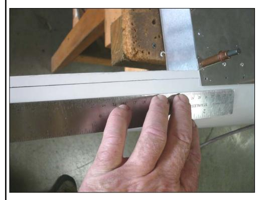
Draw a 10mm rivet line on the Stabilizer End Caps to the aft end. Layout the rivets on the line using pitch 40mm.
