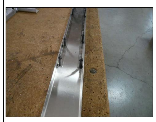
Cleco the Front Spar Cap to the Spar with 5/32 clecos.
