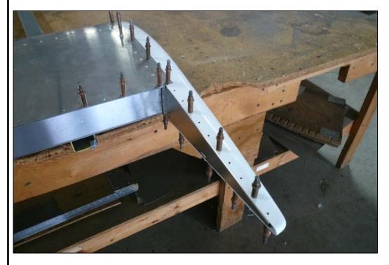
Wait to rivet the Tips on until after the Stabilizer is mounted on the Fuselage. The Tips will be removed and a level mounted on the End Rib to level the Stabilizer.
