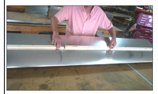
Use a furring strip (1x2 board) to bring the Skin down on the skeleton. Using ratchet straps will also help in holding the Skin down.
