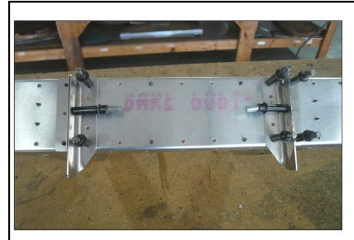
Front Spar Attachment and Attachment Doublers clecoed to the Front Spar.
