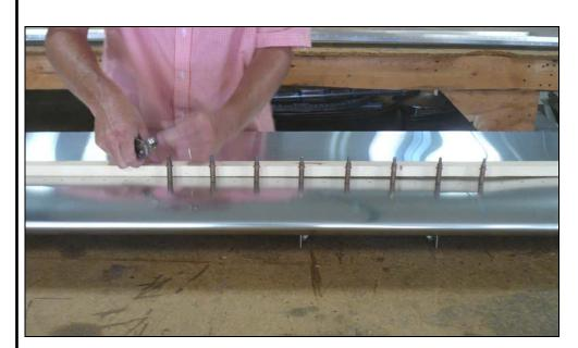
Start to cleco from the center and work out left and right. It will take a few holes to cleco before the Spar and Skin will line up.
