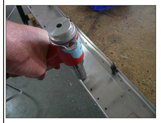
Deburr the lower Doublers and rivet the Rear Spar Bottom Doublers. At this time the top Doublers will not be riveted because the piano hinge will have to be position. Make sure not to rivet the holes where the ribs are located and in the center for the Rear Spar Attachment Bracket.
