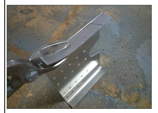
P/N: C75T2-3 Rear Spar Attachment Bracket
