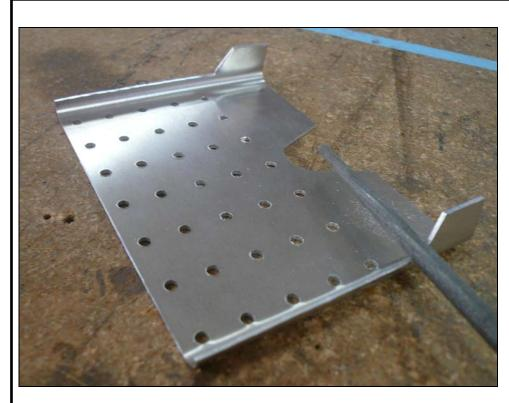
Use a hand file to remove the snip marks and even out the sides. A round file is needed to touch up the corners.
