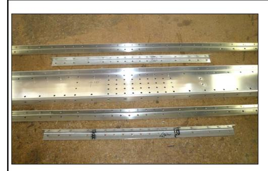
First step is to Deburr all the parts on the Stabilizer before assembly.
