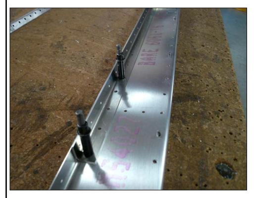
P/N: C75T1-9 Rear Lower Spar Cap
