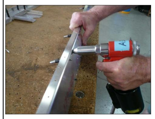
Rivet the Front Spar Cap to the Spar with A5 rivets. Do not rivet in the area for rib location and Front Spar Attachment Brackets.
