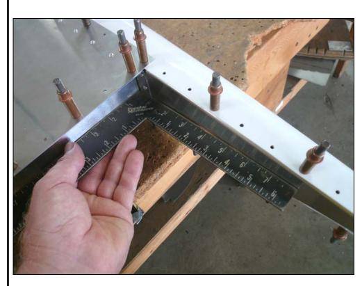
Before drilling check that Rib is square to the Spar. Drill and cleco Cap to the Rib with number 30 drill.
