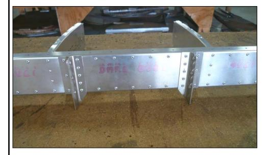
Rivet the Brackets and Doublers to the Front Spar using A5 rivets. Using a hand riveter is very helpful in this location.
