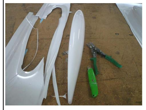
Trim Stabilizer End Caps and remove the excess material using snips and utility knife.
