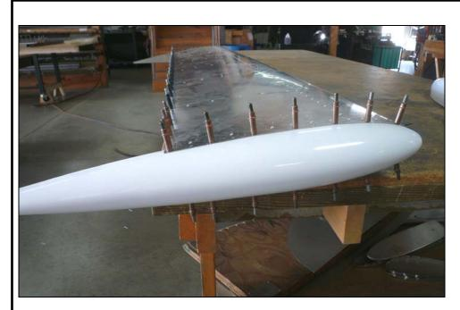
Position the Stabilizer End Cap on each end. Drill and cleco with 1/8 cleco.
