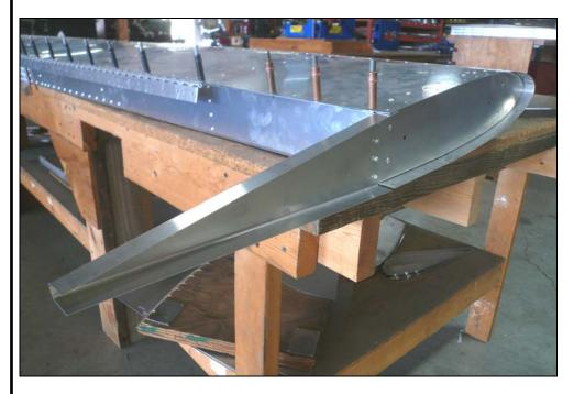
Rivet the Tip Rib using A4 rivets.
