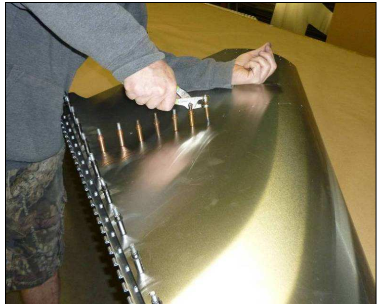
Push down on the skin and cleco the nose rib.
