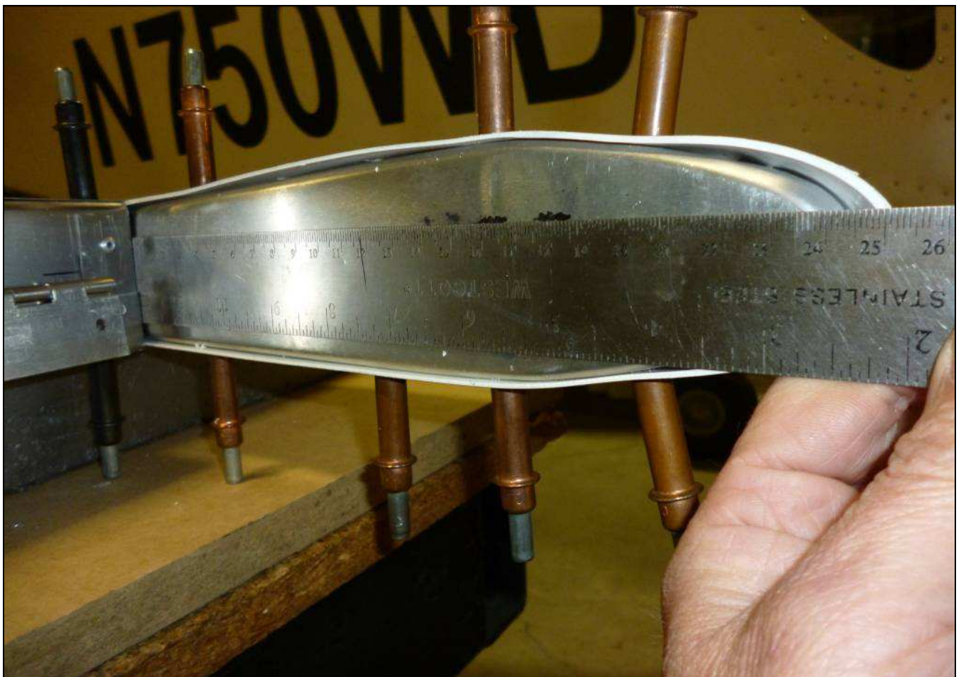
The distance from the spar to tip is 253mm ref. C75-RA-1
