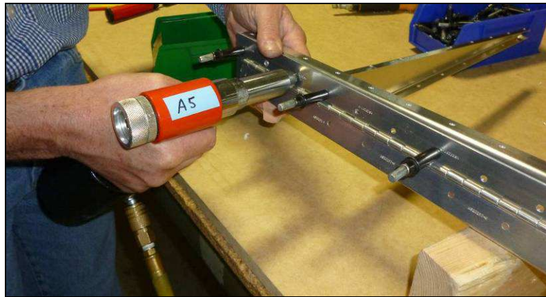
Rivet with A5 rivets.
