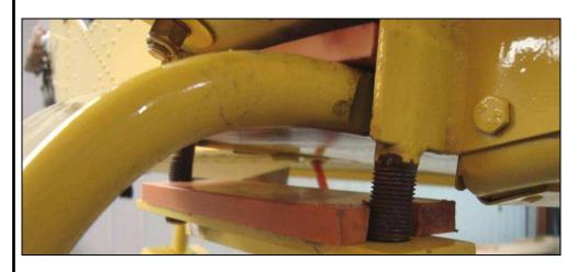
**P/N:** C75L2-2 Main gear support rubber (LOWER)
