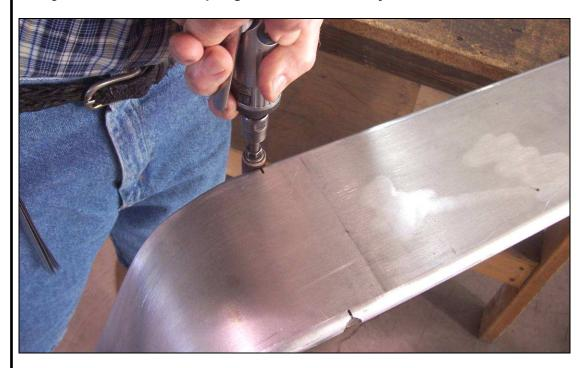
With a die grinder or rotary tool, sand an 1/8" notch into the Gear Spring for each Stud location.
