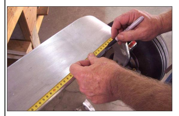
Divide the distance between the studs on the Gear Strut Fittings by two. Mark a line on the Gear Spring for the studs on the Gear Strut Fittings.
