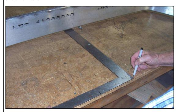
Set a square flush with the edge of the work bench on the center mark. Mark the center line on the aft side on the bottom of the Gear Spring.
