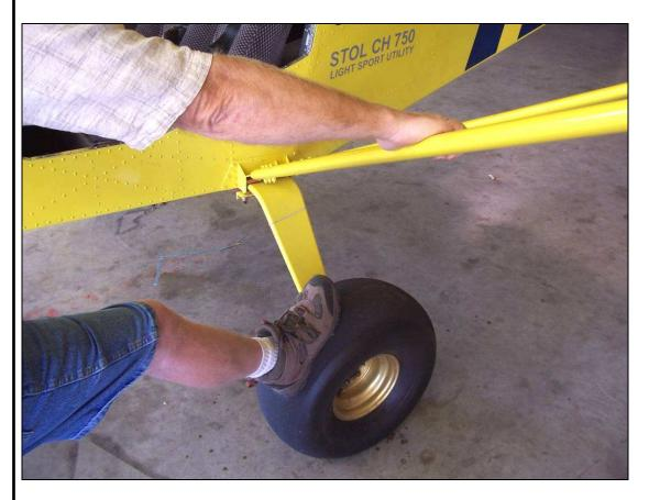
Check to be sure the Gear Spring doesn't rotate after tightening the nuts. If the Gear Spring rotates tighten the nuts further and check again.
