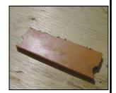
Notch the Support Rubber to clear the Studs on the Gear Strut Fittings. The notches will be centered on the bottom Support Rubber. The top Support Rubber notches will be offset to one side, see photo to the right.
