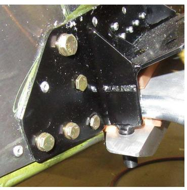
Install a washer under the lock nuts on the Studs and tighten the nuts. The nuts should be tight but should not bottom out on the shoulder of the bolt.
