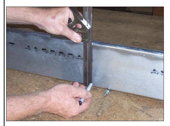
Use a smaller square to draw the center line across the Gear Spring.
