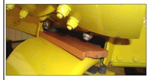
P/N: C75L2-2 Main gear support rubber (UPPER)
