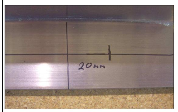
Mark a center line on the flange of the Main Gear Support. Extend the marks for the Stud locations across the center line. Drill the holes out to ½" and deburr the holes. Mark a line 20mm from the center of the hole and trim off the excess material from the Main Gear Support.
