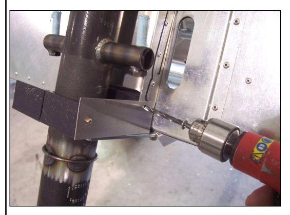
Use an AN3 bolt at the front of the Bearing to hold the drill guide in place. Set the bottom of the drill guide on the Lower Bearing Support and overlap the outside of the Center Firewall Stiffener. With a #12 drill bit, back drill through the drill guide into the Center Firewall Stiffener. Bolt the two halves of the Bottom Bearing together and to the Center Firewall Stiffener.
