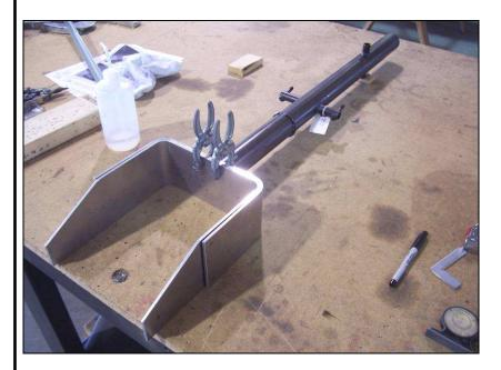
Be sure the front of the Nose Gear Leg is clamped to the front of the Fork. The tapered side is forward on the Fork and the plate to retain the bungee is on the back of the Nose Gear Leg.
