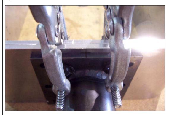
Mark the center line on the bottom plate of the Nose Gear Leg. Align the center line on the Doubler with the center line on the Nose Gear Leg. Position the edge of the Nose Gear Leg plate on the line 5mm from the edge of the Doubler and Clamp the Nose Gear Leg in place.
