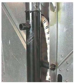
Check that the Bungee Pin is installed before installing the bottom bearing.
