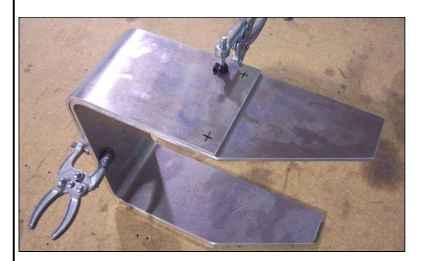
Clamp the Doubler on the Fork. Mark bolt locations 12mm from the front and back edges and up 12mm from the bottom of the Doubler on the left and right side. With a #40 drill bit, drill and Cleco the Doubler to the Fork. Expand the holes to 1/4". Deburr the holes and bolt the Doubler to the Fork with AN4 bolts.
