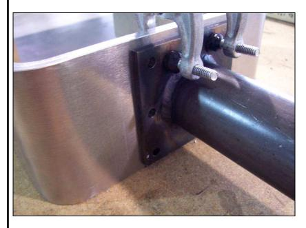
Layout 3 bolts locations on each side of the Nose Gear Leg plate and drill the holes to 1/4". Start with a #40 drill and work up to 1/4". Deburr the holes and bolt the Nose Gear Leg to the Fork and Doubler.
