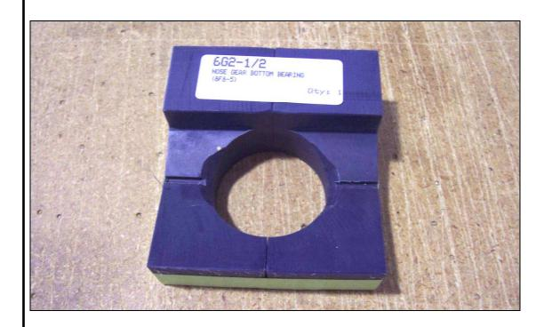
**P/N:** C75L1-7 Nose Gear Bottom Bearing
