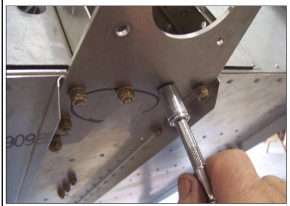
Cleco the Lower Bearing Support to the Floor Stiffener and Cabin Floor With a #12 drill bit, expand the holes. Deburr and bolt the Lower Bearing Support to the Fuselage with 8 AN3 bolts.
