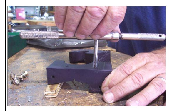
Remove the Bottom Bearing and Nose Gear Leg from the Firewall. Flip the Bottom Bearing over and use a couple pieces of plywood to support the front of the Bottom Bearing. Use a ¼"-28 tap, to tap the holes just drilled for AN4H-5A bolts. Be careful when tapping the threads; be sure the tap is perpendicular to the bottom of the Bearing.
