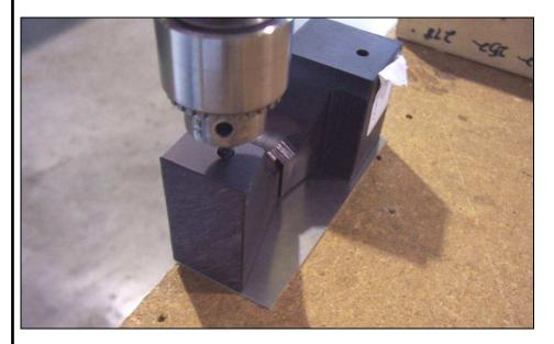
Make a drill guide for the Lower Bearing from a piece of scrap material. Be sure the scrap material is flush at the bottom and rear of the Bearing. With a #12 drill bit, back drill through the Bearing into the scrap, be sure to drill both holes.
