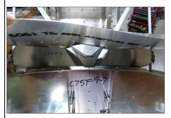
Draw a line centered on the flange of the Firewall. Also make the center of the firewall on the top flange and front of the Firewall.
