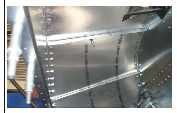
Cut L Angles to fit between the Instrument Panel and the Firewall. Draw a center line on one flange of the L Angles. Position the L Angles on the Top Skin so the center line is visible through the predrilled holes. Crimp the L Angles as required to fit the skin. With a #30 drill bit, back drill through the Top Skin into the L Angles and Cleco.
