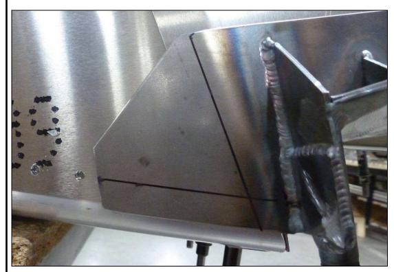
**P/N:** C75F14-3 Gear Strut Fitting
