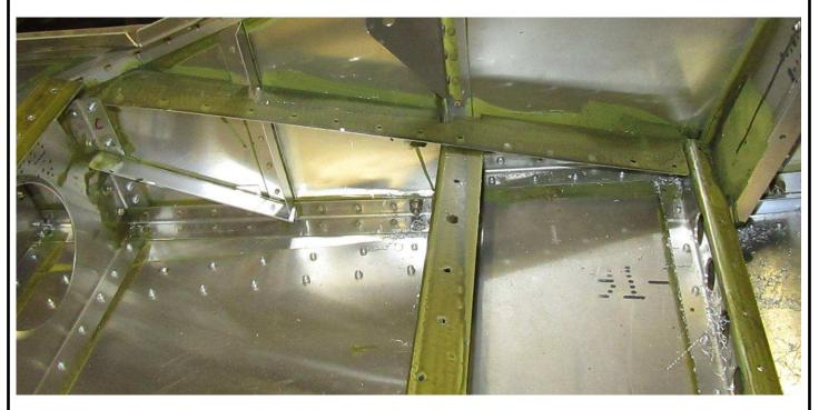
Seat base angle C75F11-7/1 (shown with the channels for the sliding seat option).
