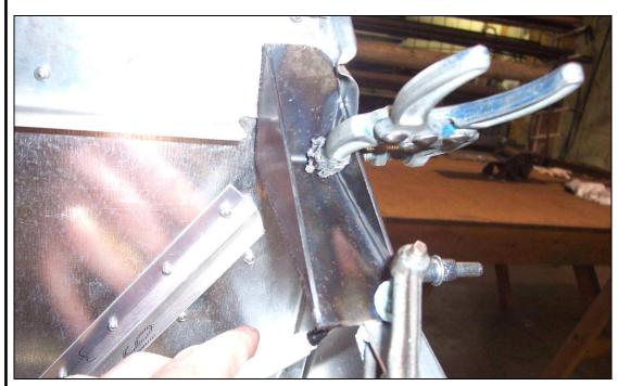
**P/N:** C75F14-2 Upper Engine Mount Fitting
