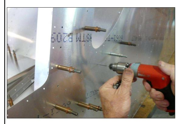
With a #40 drill bit, back drill through the Side Skin into the Longeron on the Cabin Side and Cleco. Use a #20 drill bit to expand the holes and Cleco.
