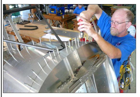
With a #40 drill bit, back drill through the Forward Top Skin into the Firewall. Start in the center and work to each edge. Cleco every hole as they are drilled to pull the Skin tight to the Firewall. Back drill through the Side Skin into the Top Skin and Longerons and Cleco. With a #20 drill bit, expand the holes for the Firewall and Longeron and Cleco. With a #30 drill bit, expand the holes through the Instrument Panel.
