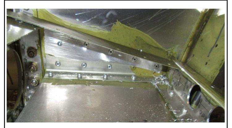
Cut a piece of L angle 150mm long. Mark the center line on one flange. Mark a rivet location 10mm from each end of the L angle, then even space 3 more rivet locations. With a #40 drill bit, predrill the holes in the L angle. Position the L angle on the Gear Channel against the Cabin Side. Back drill through the L angle into the Cabin Side and cleco. Back drill through the Gear Channel into the L angle and cleco. With a #30 drill bit, expand the holes and cleco.
