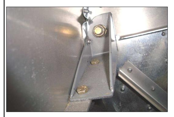
Layout a hole 10mm from the aft end of the Upper Engine Mount Fitting centered on the Longeron. Layout a hole 10mm from the front edge of the Longeron on the Upper Engine Mount Fitting centered on the Longeron. With a #40 drill bit, predrill the holes for the bolts in the Upper Engine Mount Fittings. Position the Upper Engine Mount Fitting on the Longeron, drill with a #40 drill bit, and Cleco. Expand the holes to 3/16" and Cleco.
