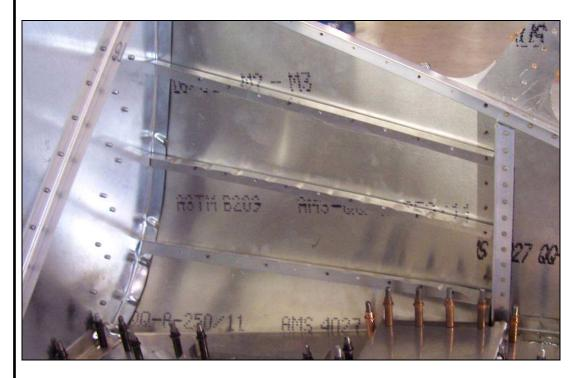
Trim L Angles to fit on the Forward Side Skin. Draw a center line on one flange of L Angles. Position the Angles on the Forward Side Skin so the line is visible through the predrilled holes. Crimp the top flange to match the curvature of the Side Skin. With a #40 drill bit, back drill through the Side Skin into the L Angles and Cleco. With a #30 drill bit, expand the holes and Cleco.
