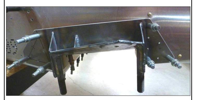
With a #40 drill bit, drill the bolt and rivet locations on the Gear Strut Fitting into the Fuselage and cleco. Expand all the holes with a #20 drill bit and cleco. Expand the 10 holes for the bolts to 3/16", then expand the top hole in the Gear Strut Fitting through the Side Channel to 1/4".
