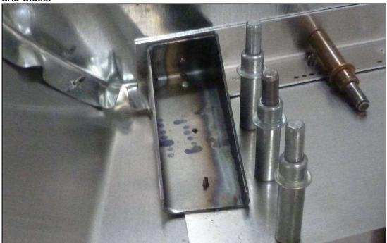
**P/N:** C75F14-1 Lower Engine Mount Fitting
