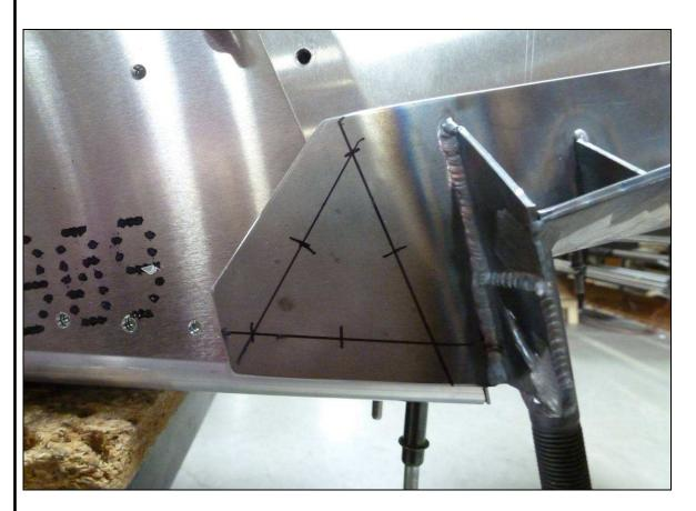
Mark a hole location 10mm from the ends and one half way between. Layout a rivet location 10mm from the edge, half way between the bolt locations.
