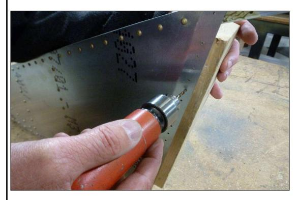
Expand the holes on the aft edge in the Cabin Side with a #30 drill bit. Use a block of wood to support the Cabin Side while drilling. Then expand the holes with a #20 drill bit.
