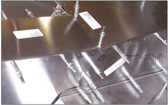
With a #30 drill bit, expand the holes in the Arm Rest Sides into the Control Tunnel Sides and Cleco.
