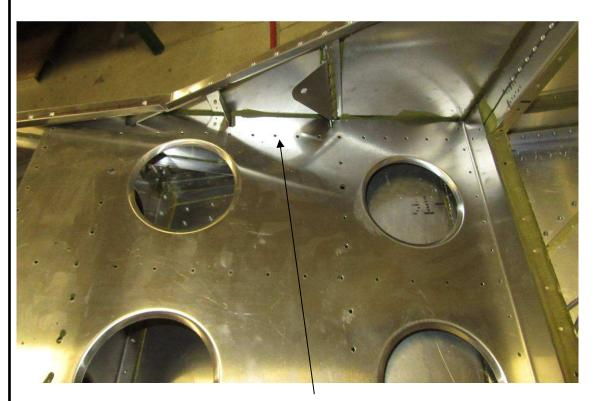
Drill the rivet line through the seat base angle C75F11-7
