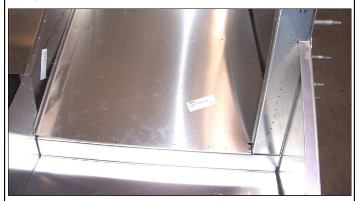
The Seat Base is positioned under the Lower Baggage Floor. With a #40 drill bit, back drill through the Lower Baggage Floor into the Seat Base and Cleco. Expand the holes with a #30 drill bit and Cleco.
