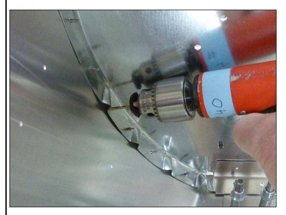
Clamp the Firewall to the Cabin Frame at the top center of the Firewall. Use a #40 drill to back drill through the flanges of the Firewall into the Forward Side Skins and cleco. Then expand the holes with a #20 drill and cleco.
