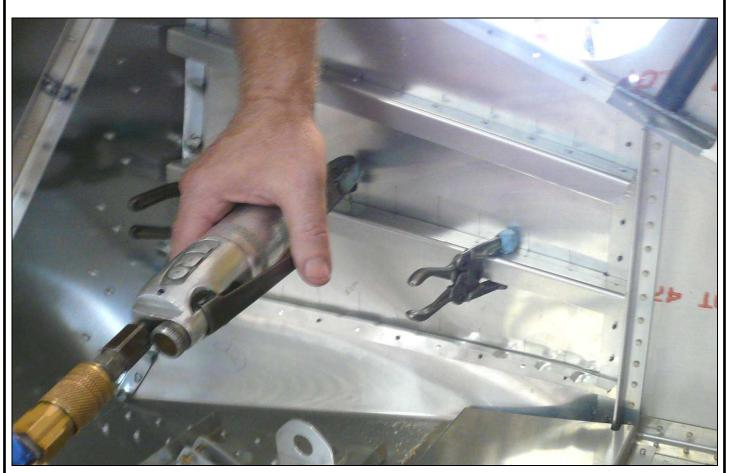
Mark the crimp locations in the L Angle on the Side Skin. Clamp the Forward Angle to the L Angle. Layout a 40mm rivet pitch making sure to miss the crimps in the L Angle, 10mm from the edge of the Forward Angle. With an Angle Drill and a #40 drill bit, drill the rivet locations in the Forward Angle into the L Angle and Cleco. Use a #30 drill bit to expand the holes.
