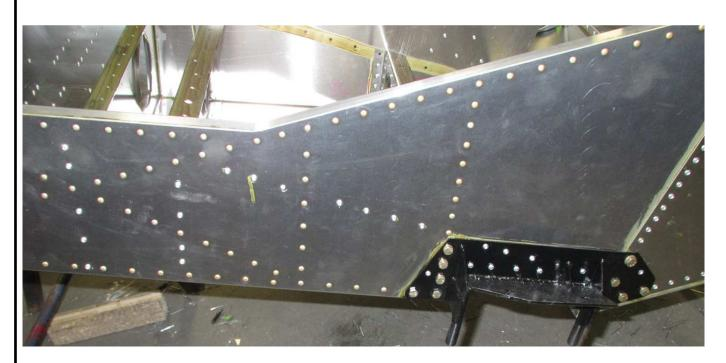
Rivets through the gear strut fitting are pulled from the inboard side.
