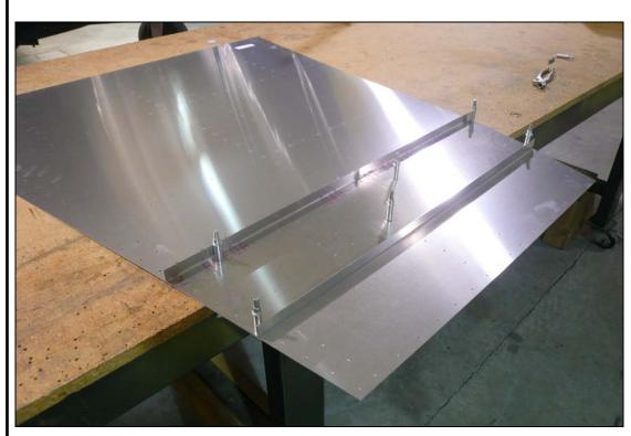
**P/N:** C75F10-7 Pedal Bearing Channel
