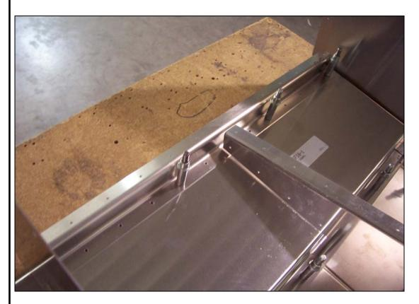
Cleco the Rear Seat Channel to the Gear Channel.
