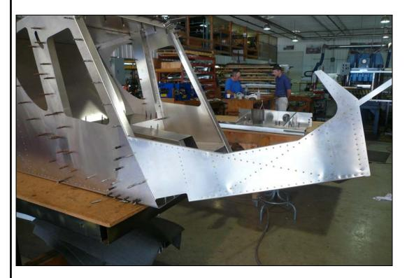
Position the Cabin Side on the Rear Fuselage. Cleco the rear rivet line to the Side Skin.
