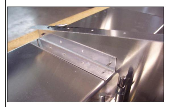
Cut two pieces of L angle 150mm long. Position the L angle flush with the front of the Gear Channel against the Seat Support and clamp the L angle to the Seat Support. With a #40 drill bit back drill through the Seat Support into the L angle and Cleco. With a #30 drill bit, expand the holes in the L angle and Cleco.
