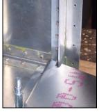
**Note:** The notch in the Heal Support should align with the vertical stiffener on the Cabin Side.
