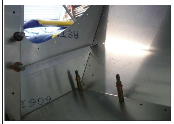
Check the length of the Longeron at the Baggage Back. If required, trim the Longeron to fit against the Baggage Back.
