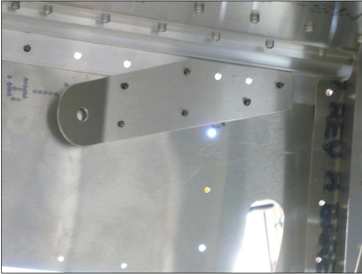
Cleco the Shoulder Harness to the Longeron and Side Skin.
