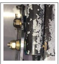
Insert the AN3 bolt through the Elevator control tube , add a 1/4" washer, the bellcrank, another 1/4" washer, then a 3/16" washer and the castle nut + cotter pin.
