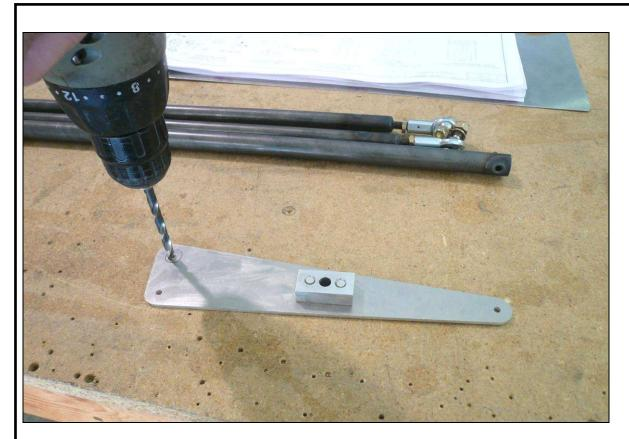
Use a ¼" drill bit to open the bottom forward hole in the Elevator Bellcrank. The bottom forward hole is located approximately 121mm from the pivot hole in the center of the Bellcrank. See drawing C75-C-2 for specific details.
