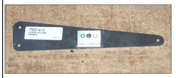
**P/N:** C75C2-6 Elevator Bellcrank
