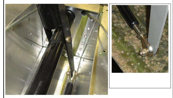
Position the Stick in a comfortable location for the neutral position.
