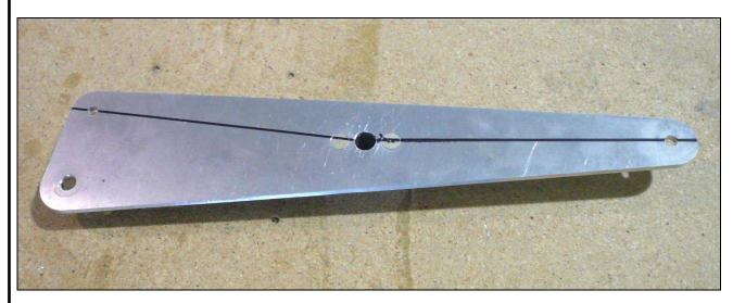
Draw a line between the Control Cable attachment holes and the Bellcrank mounting hole.
