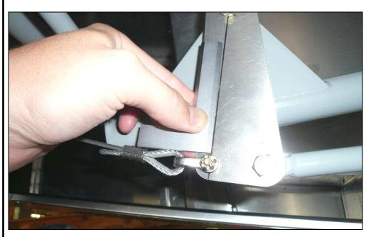
Attach the control cables to the Control Horns on the Elevator. Set the Elevator in the **Neutral** position (the top of the Elevator should be parallel to the top of the Horizontal Stabilizer). When the Bellcrank is in the Neutral position, the cable will be 90 degrees to the line on the Bellcrank. Adjust the cable length and set the Bellcrank in the neutral position.
