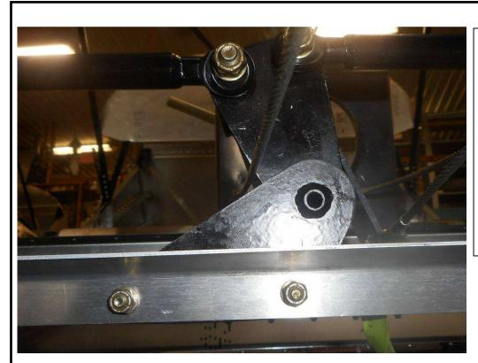
Insert the tube through the hole in the torque tube.
