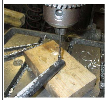
With a #12 drill bit, drill through the bushing welded to the control tube.
