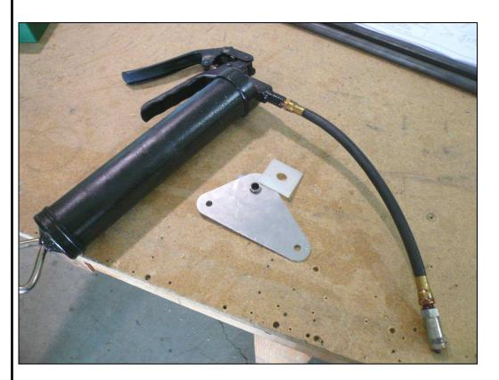
The Flaperon Bushing should turn freely in the Bellcrank, make sure the hole is large enough for it to turn but not be too loose. Grease the outside of the Bushing and the faces of the Bearings that contact the Bellcrank.
