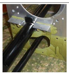
On the aft side, the Flaperon stops C75Z1-12 are bolted Through the AN3 bolts (ref. DWG C75-ZA-6)
