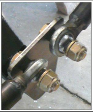
Install the Bolt on the Torque Tube. Slide the first Rod Bushing on the bolt, followed by the Control Rod and a second Bushing. Tighten the nut and properly torque the nut on the bolt.
