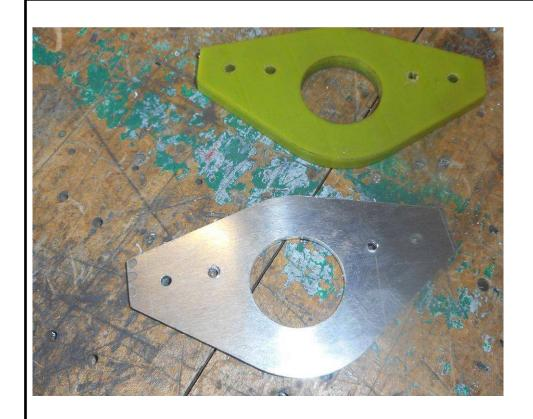
**P/N:** C75C2-3 Rear Torque Tube Bearing
