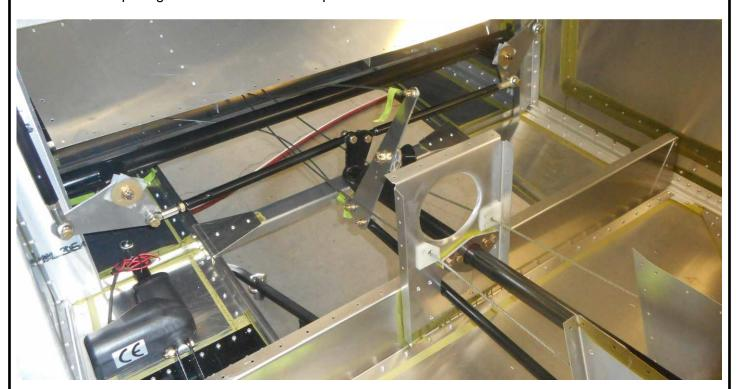
The 15mm x 20mm plate welded on the Torque Tube Bearing is against the Bearing Support (back side)
