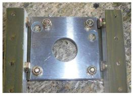
**P/N:** C75C3-1 Front torque Tube Bearing
