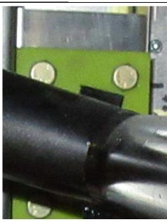
Check: The welded tab is below the bolts Note: the center of the 30.8mm hole is 30mm Up from the bottom C75C1-4
