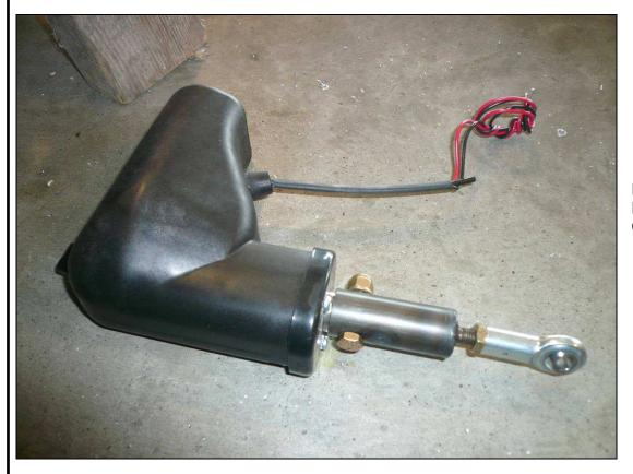
**P/N:** C75C1-3 Linear Actuator Control Rod
