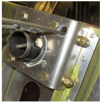
The welded tab on the torque tube make contact with the Bearing support C75F5-1. Install the Stainless Steel Shim and Stop Ring on the end of the Torque Tube.
