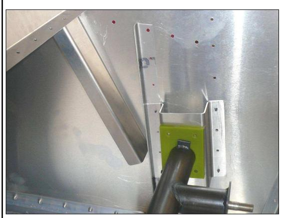
Cut an L angle 303mm long. Position the L Angle against the tab on the Longeron and against the inside of the Bearing Support. Clamp the L Angle to the Bearing Support. With a #40 drill bit, back drill through the Skin into the L Angle and Cleco. Expand the holes with a #20 drill bit and Cleco.
