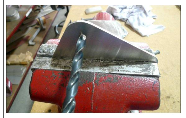
Use a  $\frac{1}{2}$ " drill bit to expand the mounting hole in the Flaperon Bellcrank. See drawing C75-C-1 or 75-CA-1 for the specific hole if in question.
