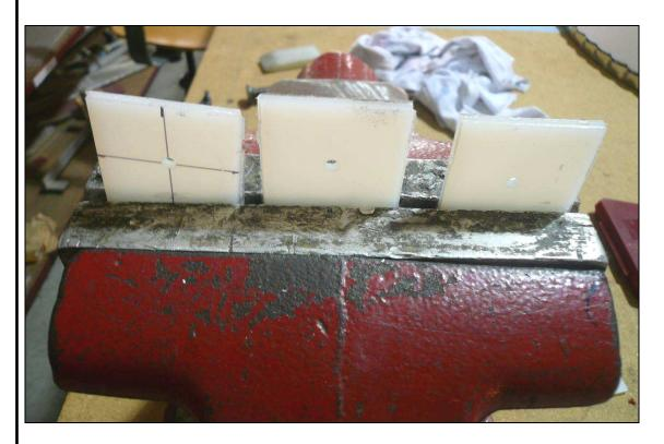
Mark the center of the Flaperon Bellcrank Bearings. With a #40 drill bit, drill a hole in the center of the Bearing. Expand the hole up to  $\frac{1}{2}$ " in steps. It is helpful to clamp the Bearing in a vise to prevent it from spinning while drilling the holes.
