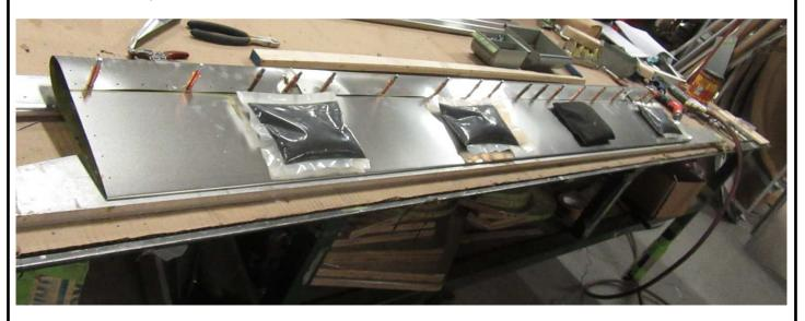
Position the weights beside the rear ribs. There should be no twist: the assembly sits flat on the workbench.
