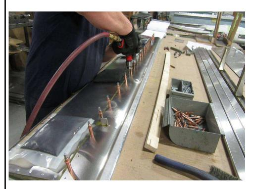
Run a #30 drill through the holes and rivet.
