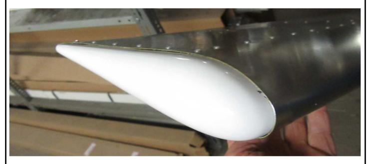
Position for the best fit by closing the gap at the front.
