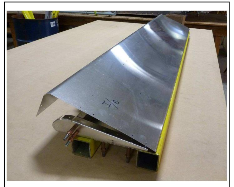
Position the assembly on beams (with clecoes in the bottom side) or on a flat workbench (without any clecoes in the bottom side as shown in the next photo)
