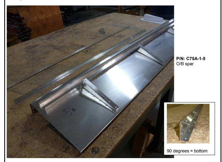
Position the ribs and spar on the skin to line up with the holes. Circle the holes for the rib on the spar web.
