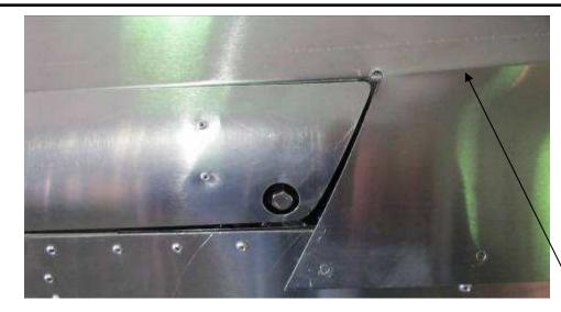
Bottom edge is trimmed just above the fuselage side.
