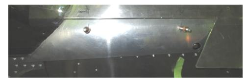
The advantage of installing the cover with just 1 rivet in the tab is that the curvature of the tap is then not critical.
