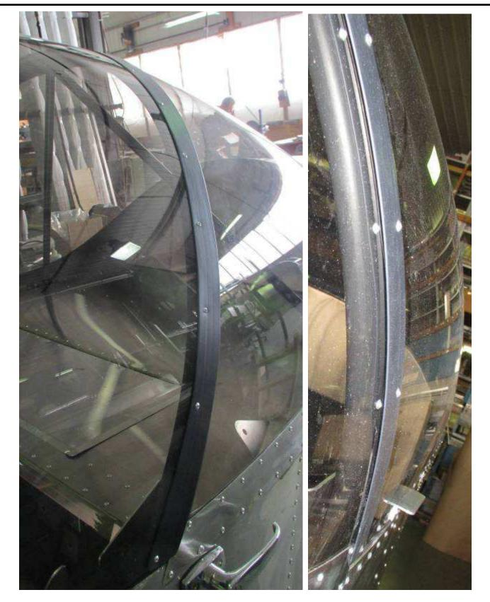
No gap on the front side. It is acceptable for the strip not to touch the rear canopy.
