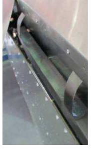
Line up the top edge. Trim the front and aft ends. Drill the hole for the bolt (big enough to insert a socket).
