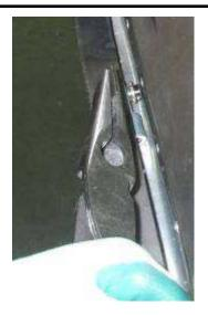
Bend the steel tabs on the canopy side frame.
