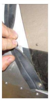
Allow 1/8" clearance of the front edge with the fuselage when the canopy is open.
