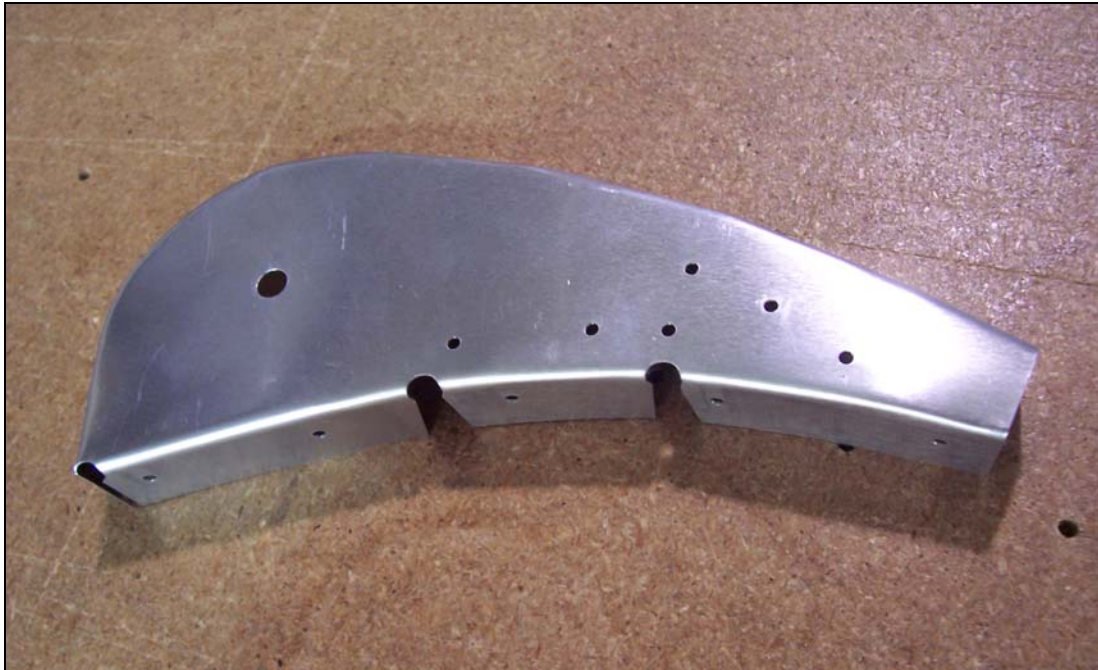
P/N: 75S1-1SS Slat Rib (predrilled for the slat support)
