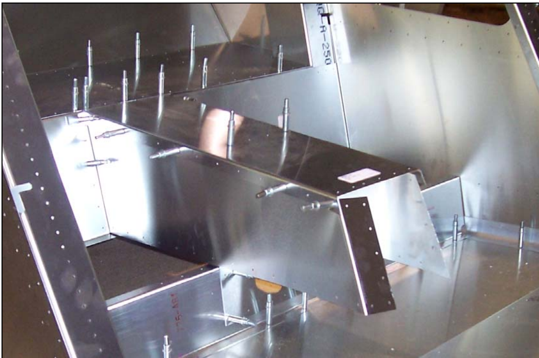
P/N: 75F6-4 Control Tunnel Top
