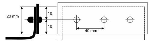
Rivet Spacing: 40 mm. = PITCH 40
