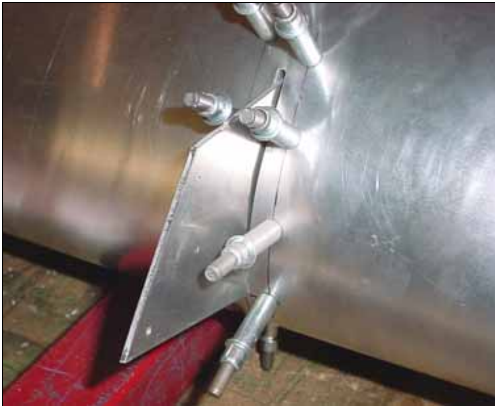
Drill and Cleco the skin to the bend L angle. Ref nose ribs #3,#4, and #6.
