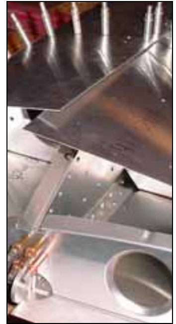
First hole is at the intersection of the spar with the rear rib #1
