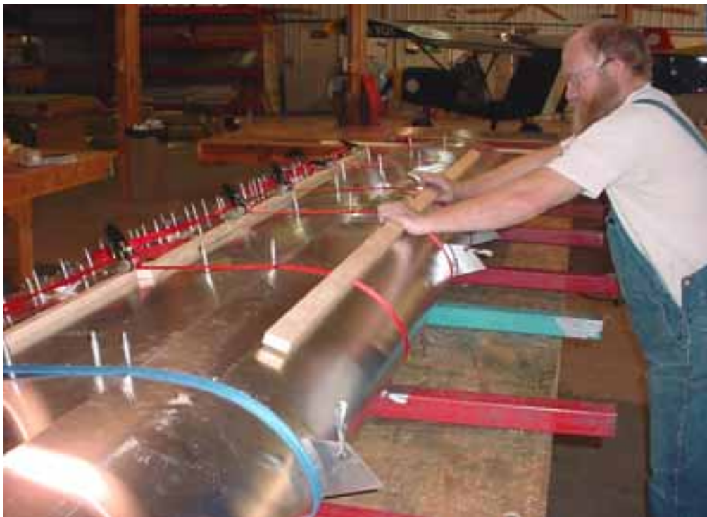
It will work better using a 1 by 2 to hold down the skin until the straps are in position and secure to the wing.
