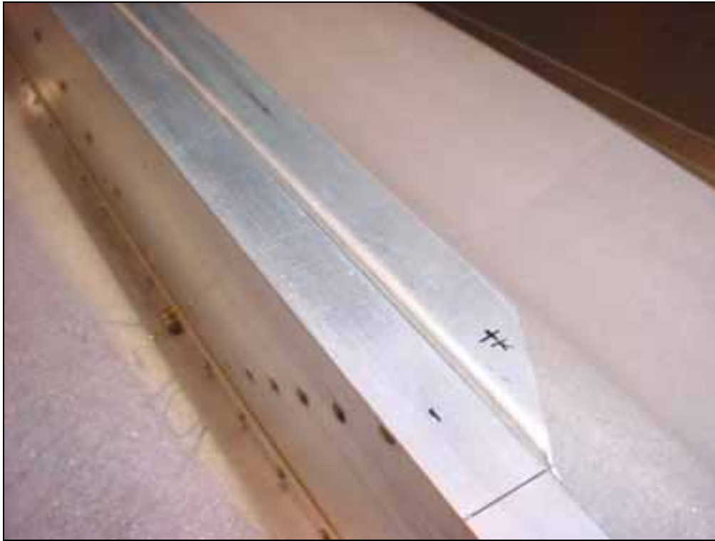
Photo looking at the top flange of the web doubler 7V2-6SP. Detail of inboard corner.
