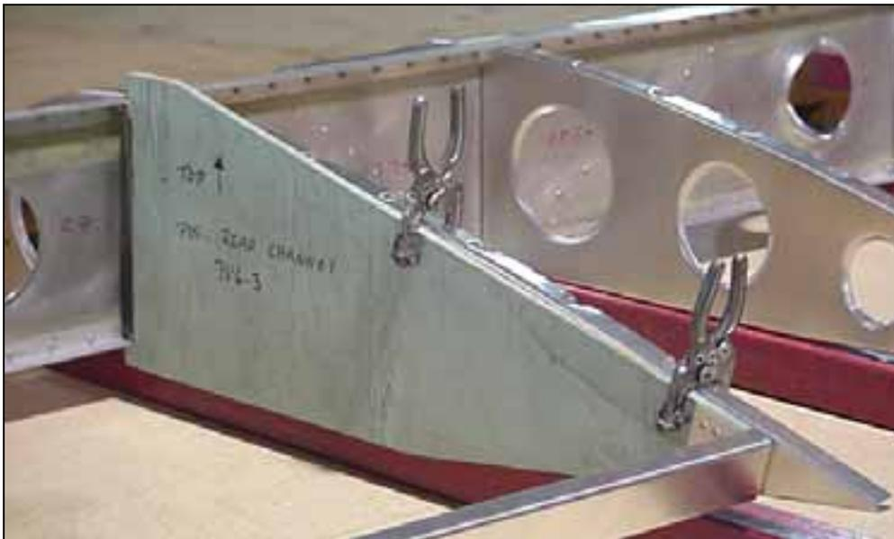
The purpose of the template is to set the distance and angle of the rear channels to the side of the rear ribs.
