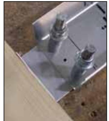
JIG: Screw the board into the workbench.
