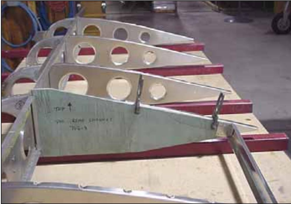
Position the template on the next rear rib, clamp to the rear rib.
