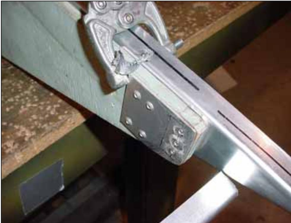
CHECK: The aft edge of the template is even with the top and bottom of the rib.
