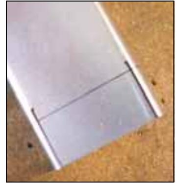
Layout the cut line along the bend tangent line on the web.
