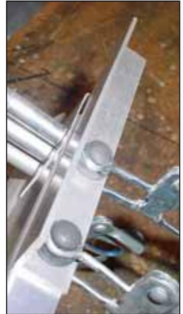
CHECK: Extrusion is even with the web (back portion of the channel – same reference used to mark the rib on page 10).
