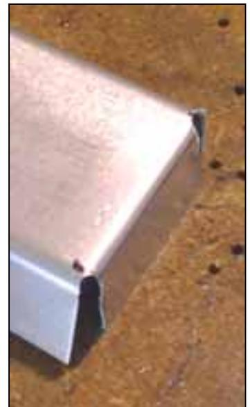
Note: The bend is in line with the corner relief holes.
