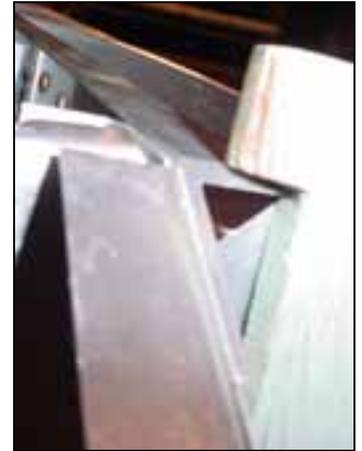
CHECK: The top of the template is pushed up against the aft edge of the upper spar cap 7V2-2 (3/4" extrusion).
