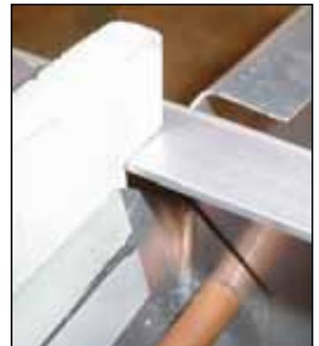
Detail: aft edge of extrusion touches the inside cutout of the template.
