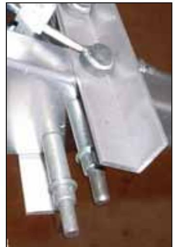
Clamp the extrusion to the rib flange.
