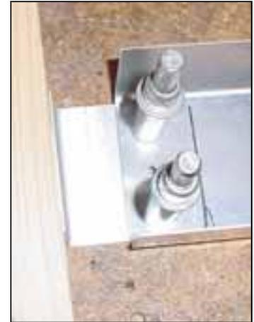
Layout 3 holes 10mm from the end of the channel.
