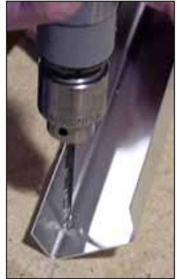
Alternative: drill corner relief holes before cutting flange.
