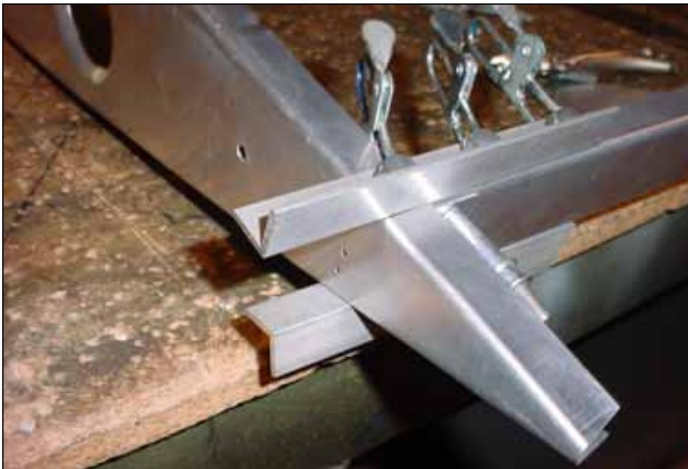
Slide the channel assembly between the top and bottom flange of the rear rib. Line up the edge of the extrusion with the lines on the rib flange (top and bottom).
