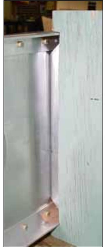
CHECK: template fits over the upper and lower spar cap 7V2-2 and 7V2-3
