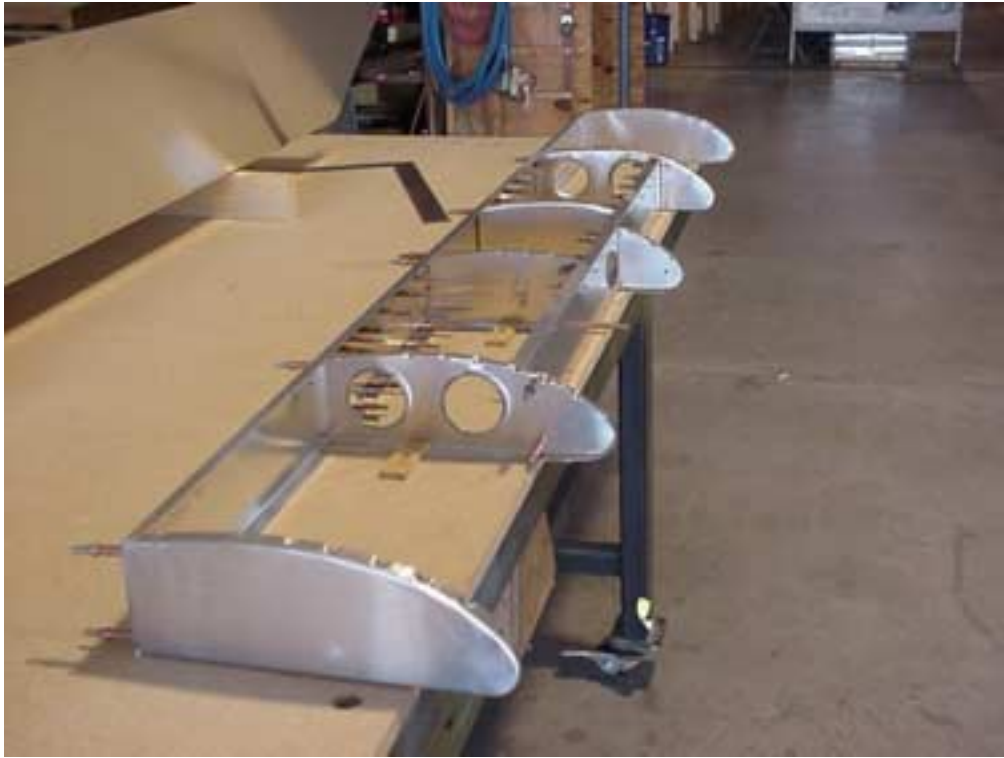
Stabilizer skeleton shown upside down on the workbench.
