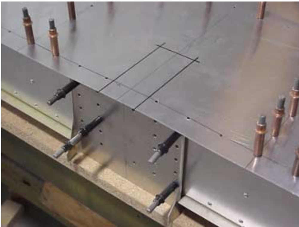
Cutout on top side only of stabilizer skin (to make room for the upper elevator cable)
