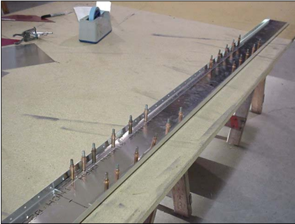
7H2-2 Rear Spar 7H2-3 Upper Doubler 7H2-5 Lower Doubler
