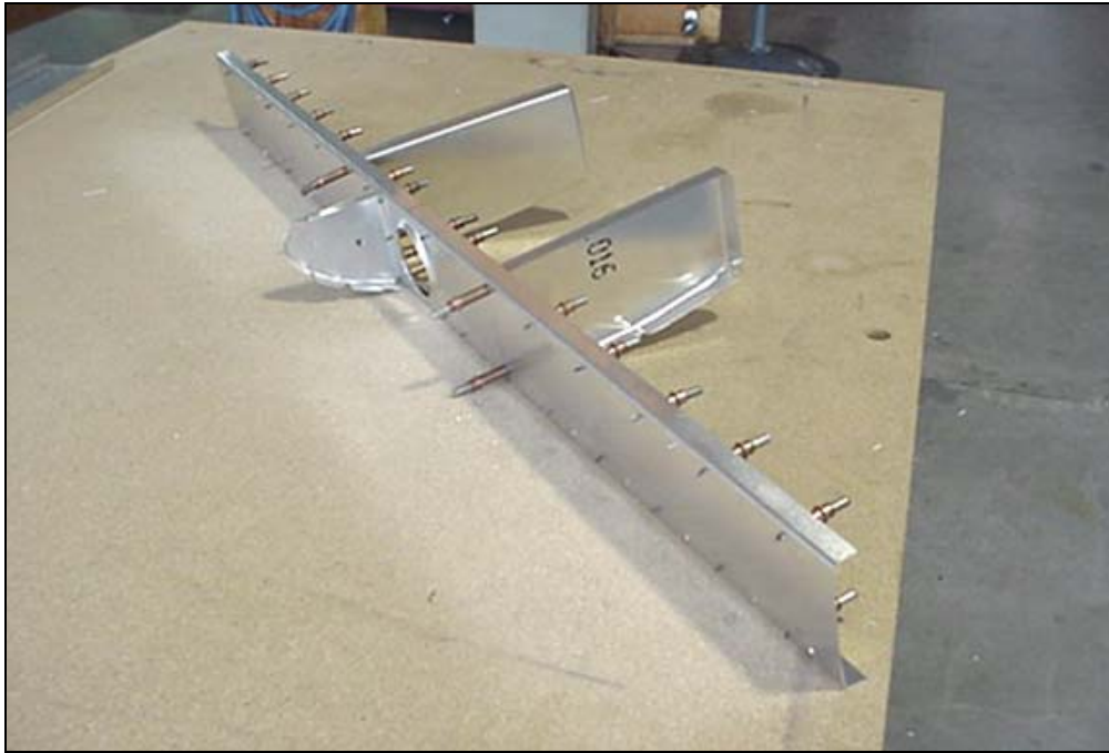
7H1-4 Rear Ribs 7H1-3 Nose Rib
