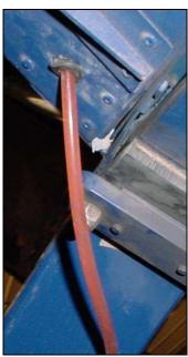
Location of grommet in cabin floor, see bottom left diagram on drawing 7-F-9
