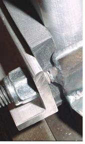
Check that the Gear Plate does not make contact with the Channel Pick (bottom of gear strut fitting). Do not over torque.
