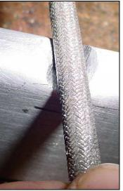
CHECK: The notch is not too tight: taper the sides of the notch to allow the gear to flex around the welded gear bolts.
