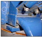
Detail gear strut fitting: The gear is firmly held in place between the top and bottom rubber spacers.
