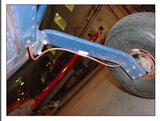
Brake line routing along the aft edge of the landing gear.
