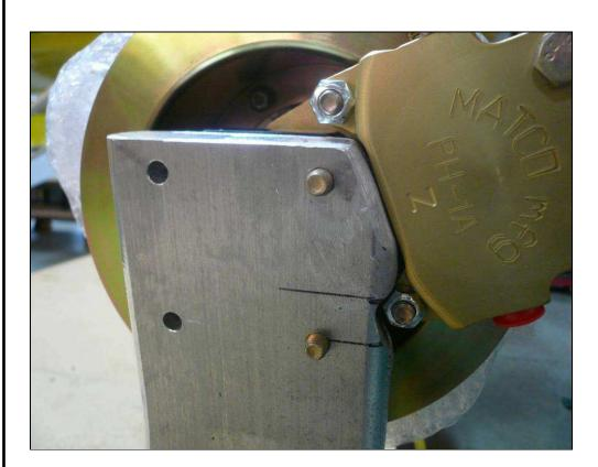
The calipers does not touch the landing gear. The caliper assembly should still be able to slide in and out without touching the gear.
