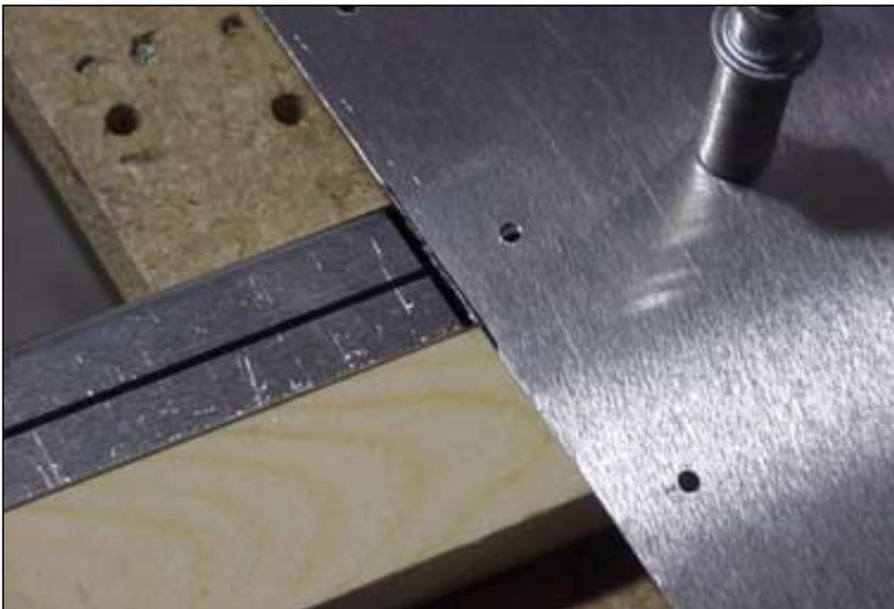
With a marker, trace along the edge of the skin to mark the length of the 'L' Angle.
