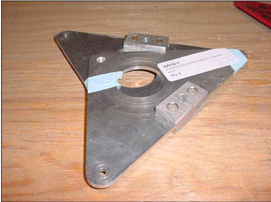
Aileron Bellcrank 6W10-1 as supplied with the Spacer 6W10-2 already riveted in place.
